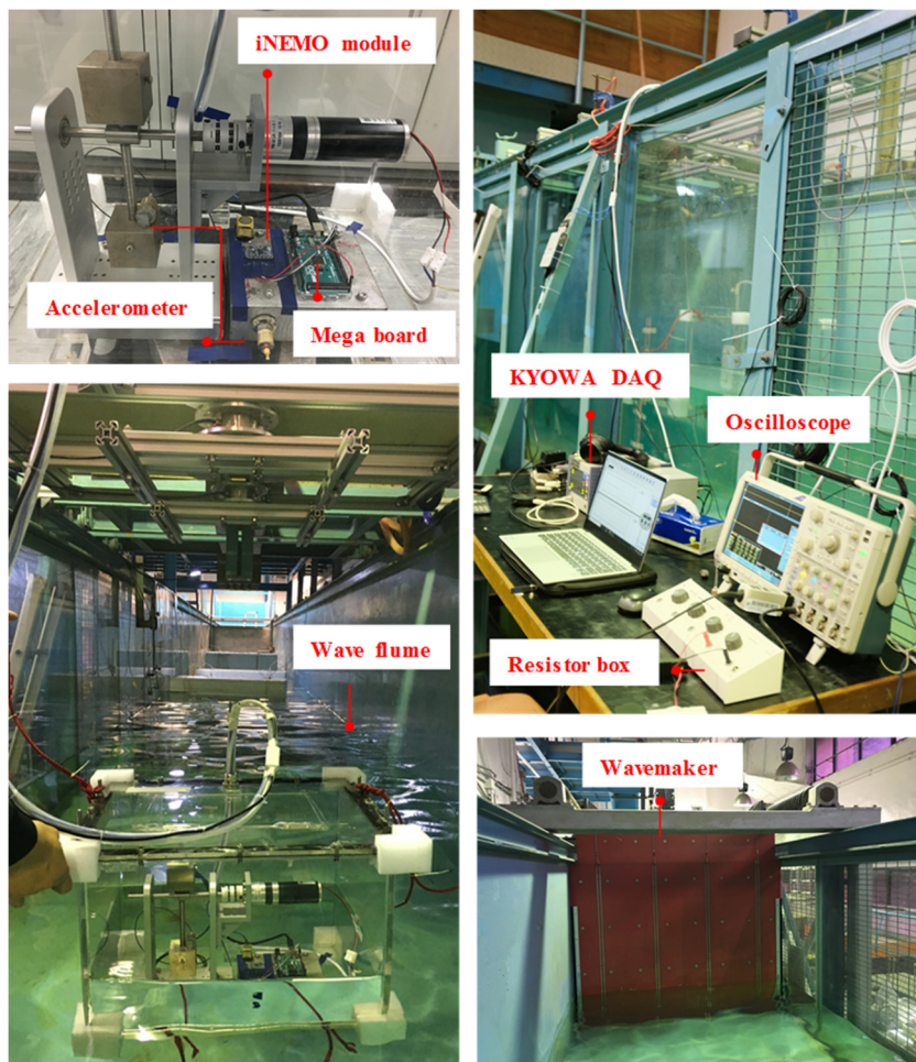
Figure 9.4 Wave flume test setup
