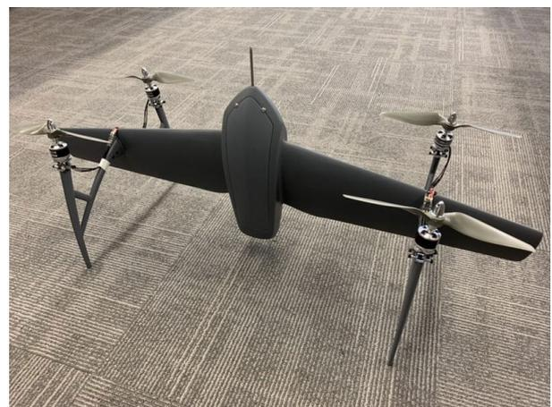
Figure 1-6 Alfa Pixhawk 2 Tailsitter VTOL [15]
