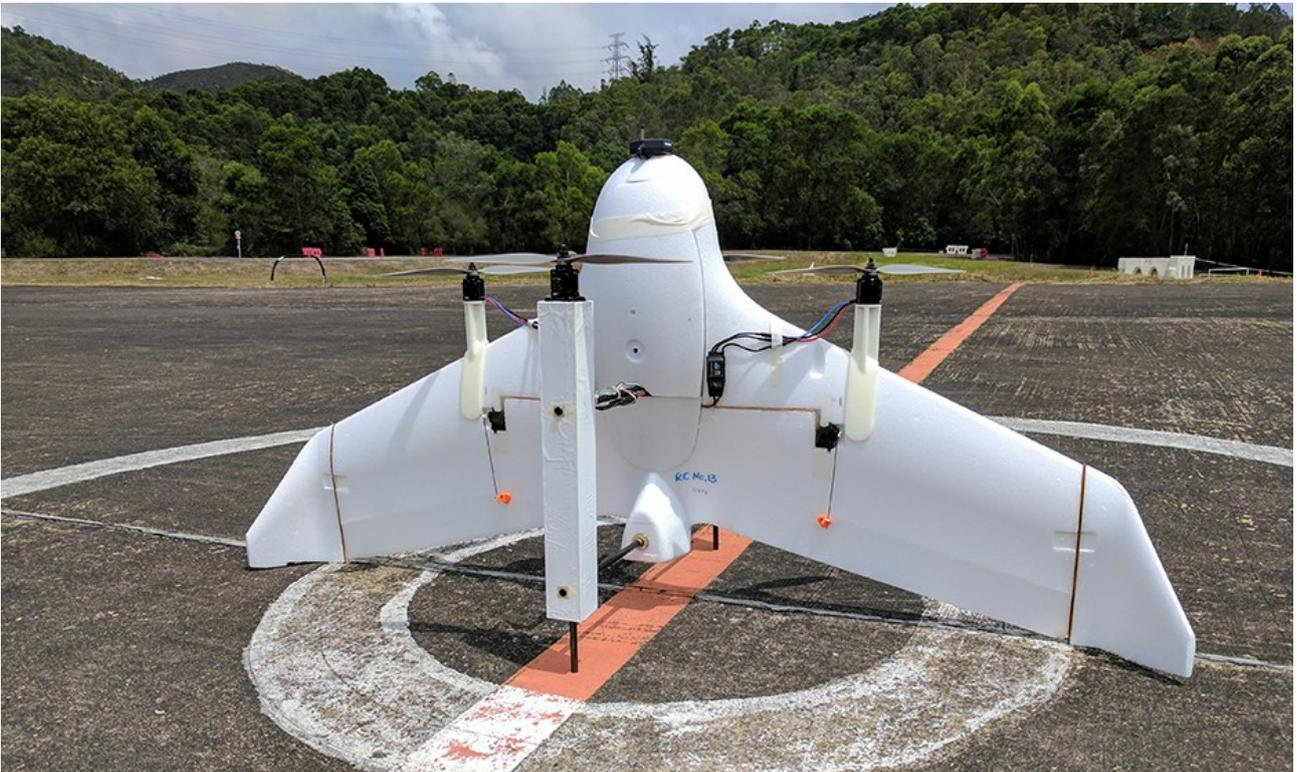
Figure 4-1 The testbed tail-sitter: PolyU Plus
