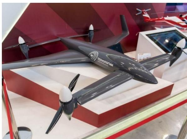
Figure 1-2 Russian Tiltrotor UAV RHV-35 [11]
