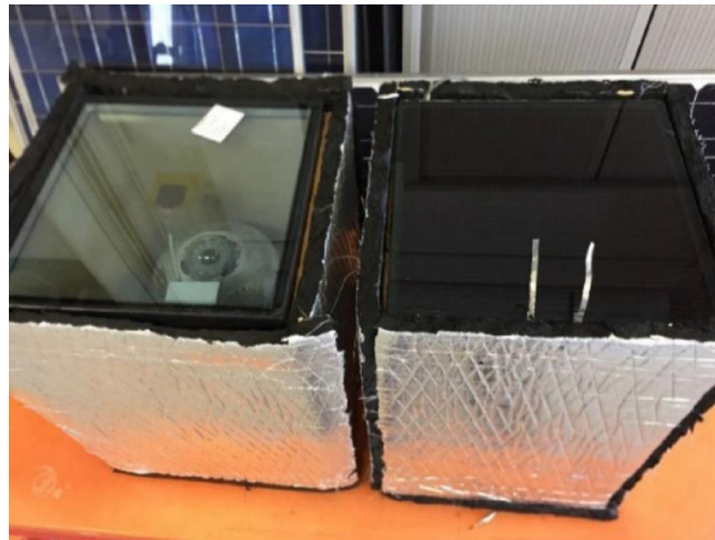
Figure 2.3 Small size hot boxes (0.3 × 0.3 × 0.4 m 3 ) (Qiu et al., 2018)
