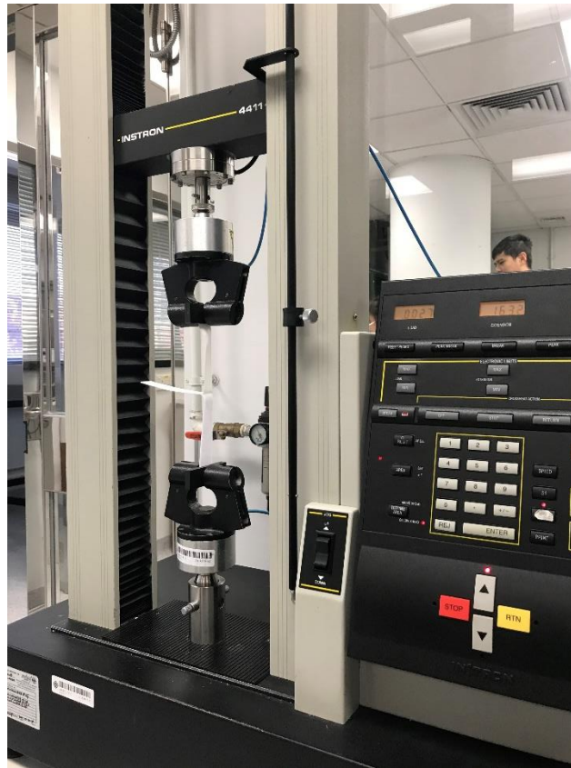
Figure 3.6 Instron 4411 tester used for peel strength test
