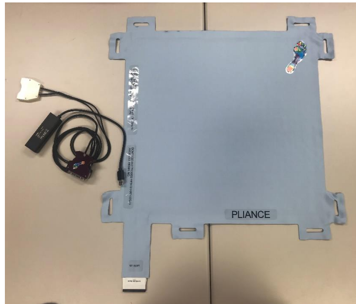
Figure 3.24 Novel Pliance pressure mat
