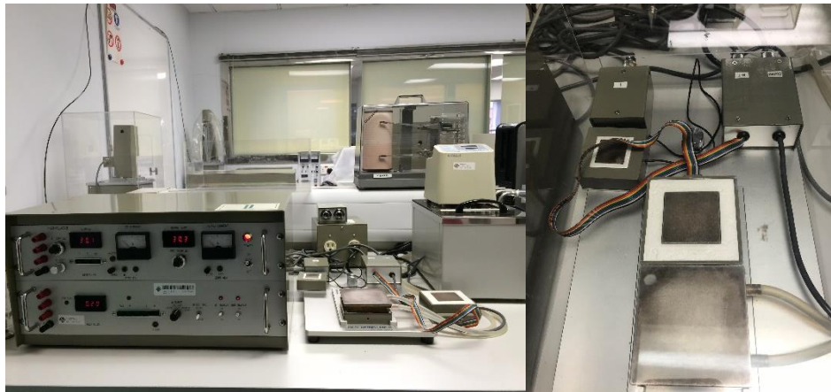
Figure 3.2 KES-F Thermo Labo II
