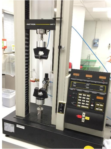
Figure 3.5 Instron 4411 Tensile Strength Tester
