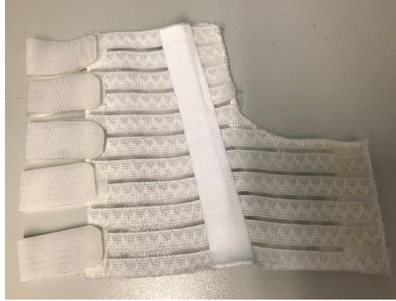
Figure 4.4 Appearance of corrective bands used in functional intimate apparel after repeated stretching
