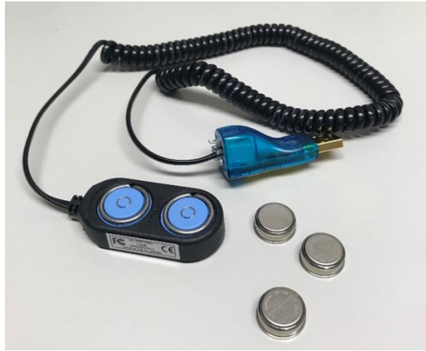
Figure 3.27 (left) Blue Dot™ receptor and (right) Thermochron™ iButton sensors
