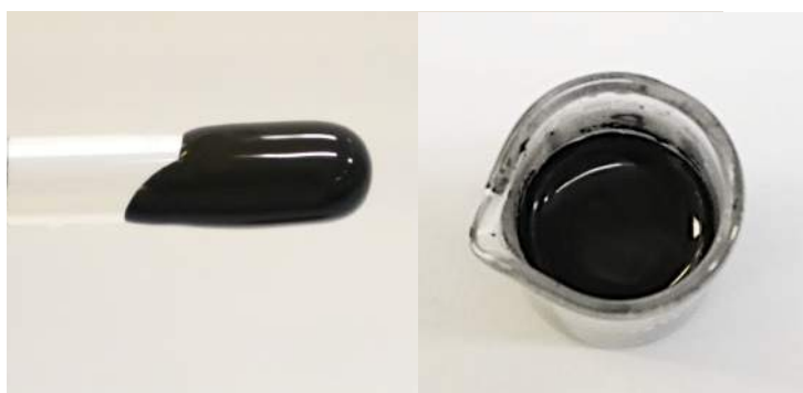
Figure 3.2 Photograph of p-type \text{Bi}_2\text{Te}_3/\text{PEDOT:PSS} ink.
