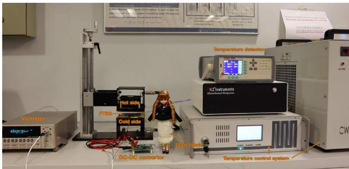
Figure 5.1 Measurement system of TEG performance
