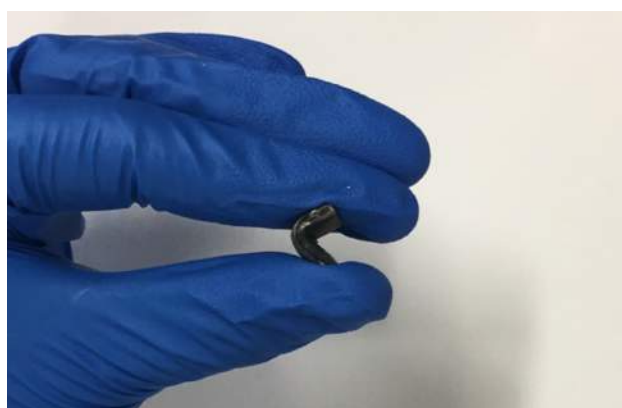
Figure 5.5 Image of 5 layers of p-Bi 2 Te 3 / PEDOT:PSS based flexible TE film.
