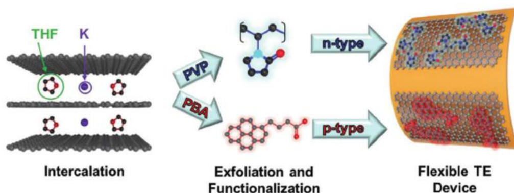
Figure 2.5 Illustrated scheme of p-type and n-type graphene films modified by changing the surfactant during exfoliation.
