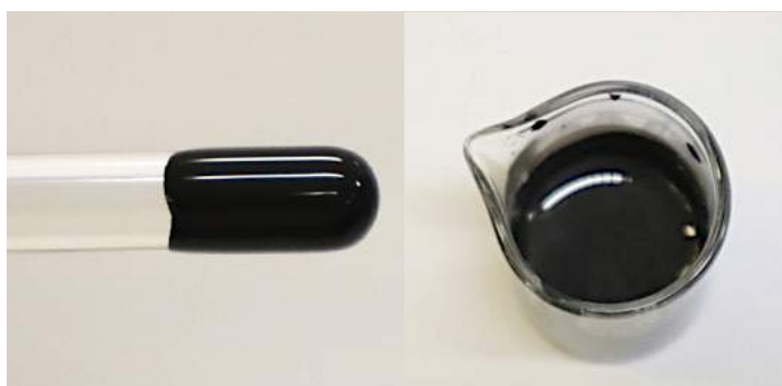
Figure 4.2 Photograph of p-type \text{Bi}_2\text{Te}_3/\text{PEDOT:PSS} ink.
