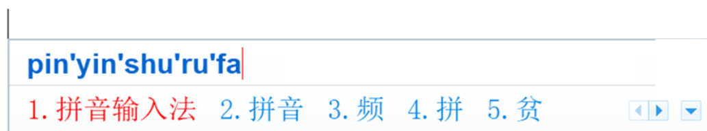
Figure 4-1 An example of the pop-up candidates box. The user input the Latin text "pin' yin' shu' ru' fa", shown on the top of the candidates box, and five corresponds Chinese words/phrases are generated automatically by the system, shown below the user input. The user can either choose the correct mapping by pressing the number key or press "space" to select the first option.
