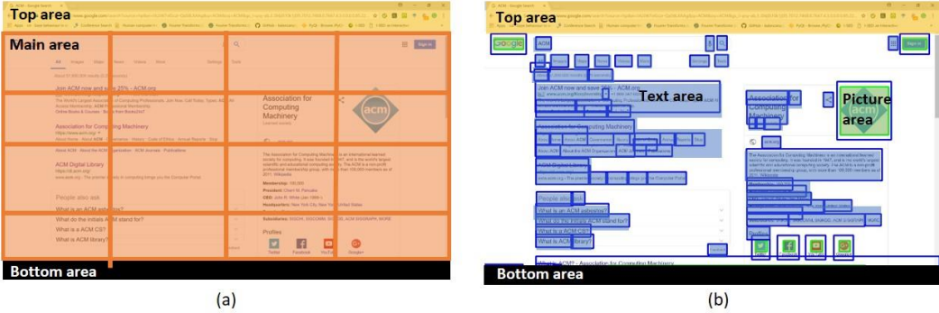
Figure 3-13 Dynamic UIs component detection methods: (a) Heuristic-based and (b) Content-based
