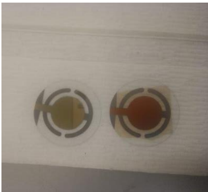
Fig.3-1 Original QCM detector (left) and coated QCM detector (right).
