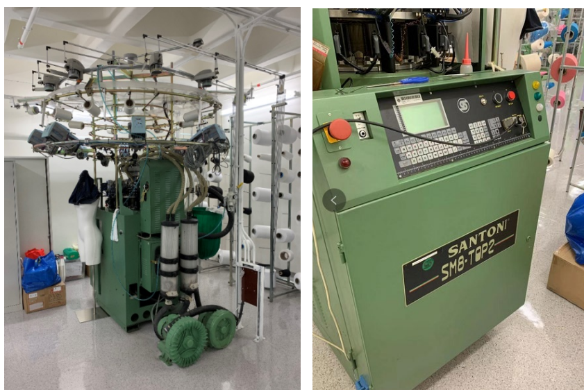
Figure 33. Santoni-Top 2 seamless circular knitting machine with 13-inch in diameters and 28 machine gauge
