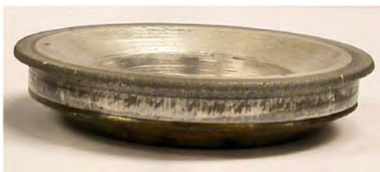
Fig. 6.38 The bimetallic component produced by warm forming.
