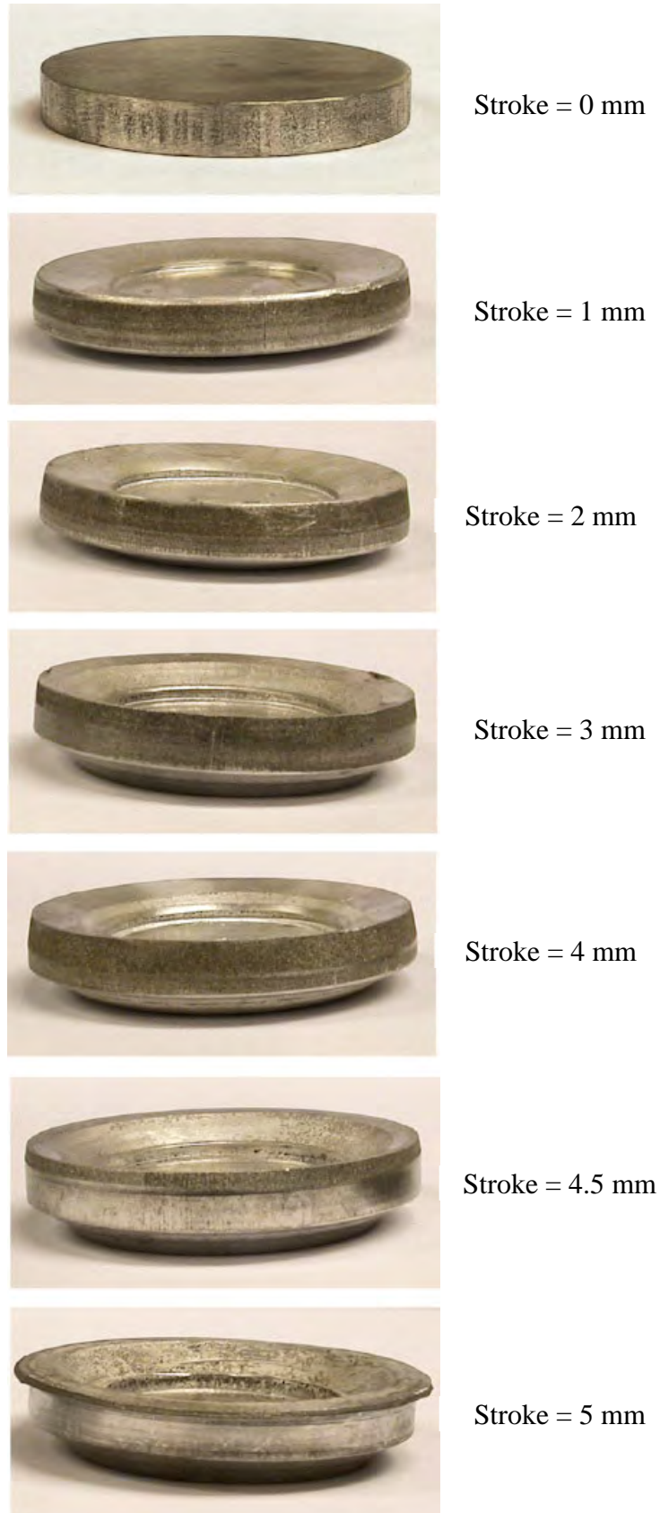
Fig. 6.26 The axisymmetric component produced by warm forming.
