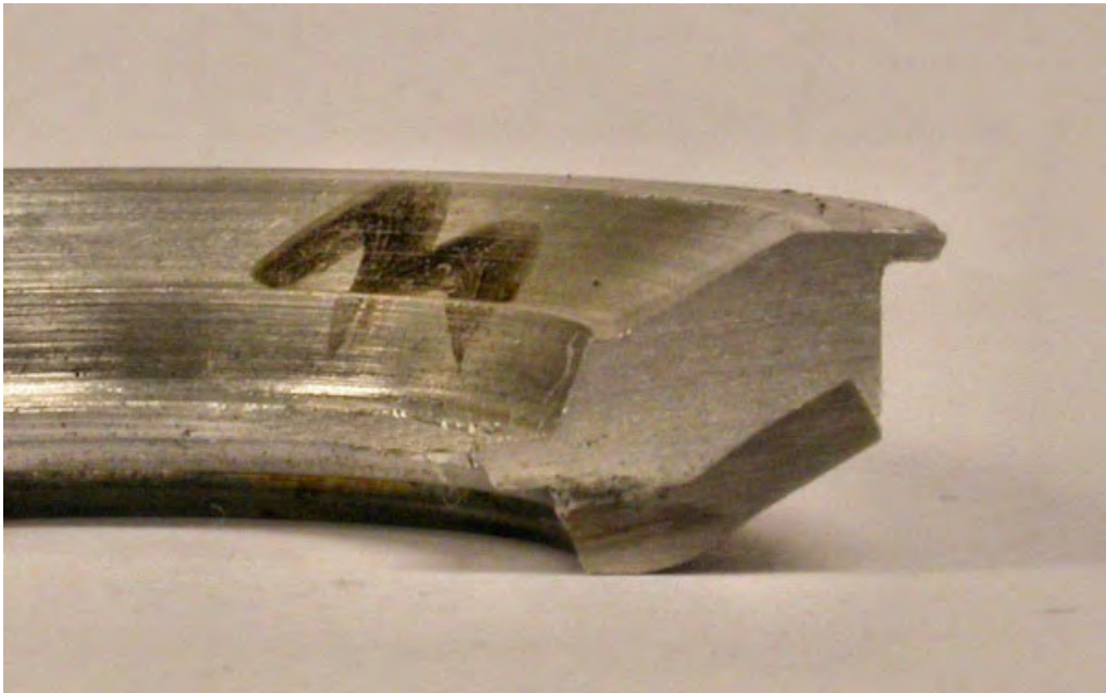
Fig. 6.40 The cross section of the bimetallic component.
