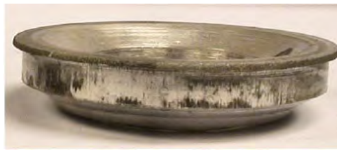
Fig. 6.32 The hollow axisymmetric component produced by warm forming.
