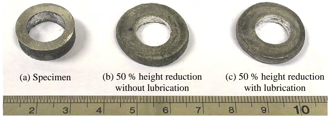
Fig. 6.1 Ring specimen and experimental results from the ring compression test.
