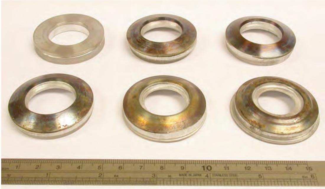
Fig. 6.39 The forming sequence of the bimetallic component.
