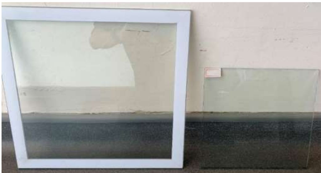
Figure 8.6 Photographs of ordinary glass (left) and ordinary glass with the spectrally selective coating
