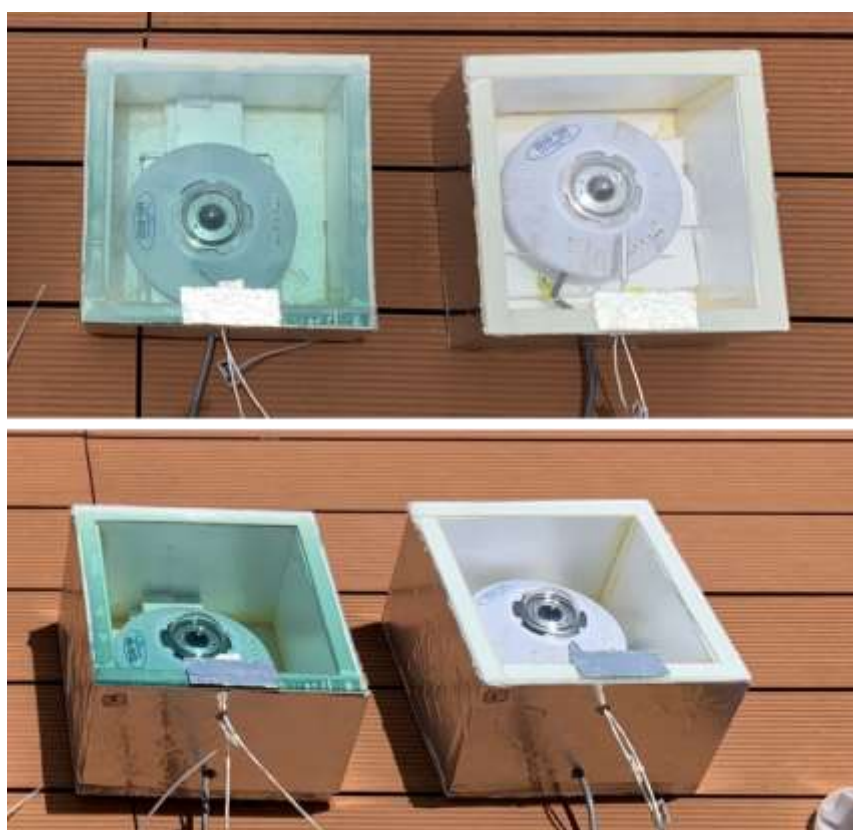
Fig. S1 Photos of top view and side view of the coated glass and ordinary glass.
