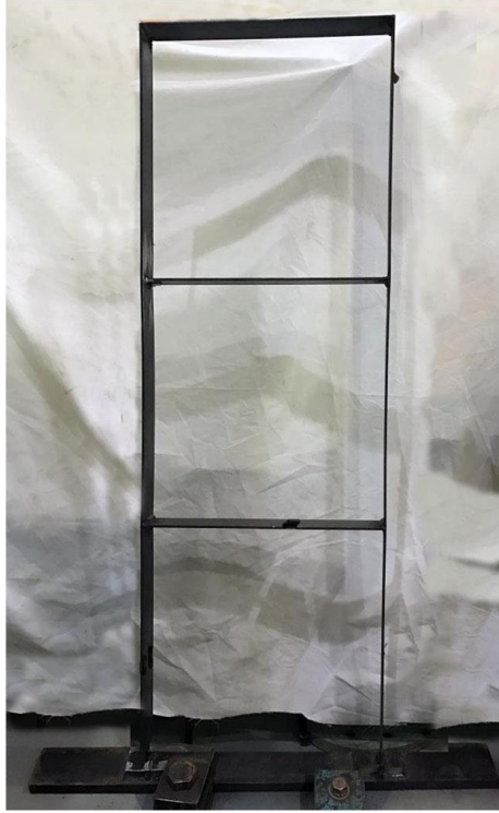
Figure 5.1 Overview of the three-story steel frame
