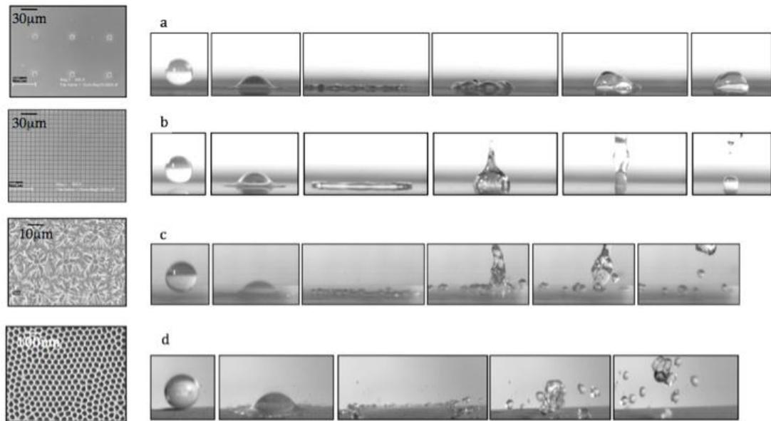
Fig. 2.21 Dynamic interactions of droplets with different surfaces. (a) microtextured surfaces with large spacing, (b) microtextured surfaces with small spacing, (c) hierarchical textured surface and (d) nanoporous surface in Varanasi's work (Varanasi, Deng, Hsu, & Bhate, 2009).
