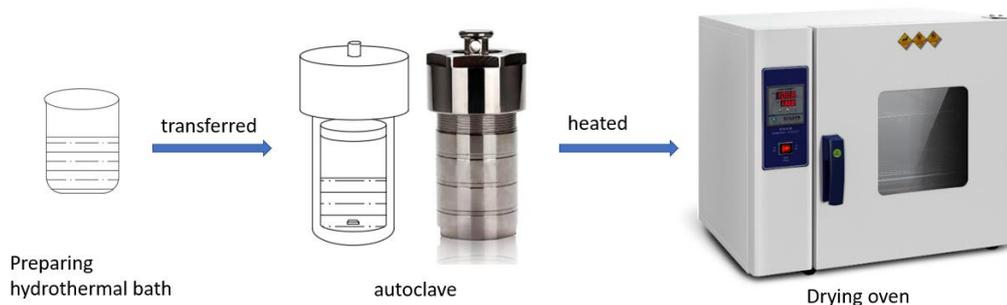
Fig. 3.3 The process of hydrothermal synthesis
