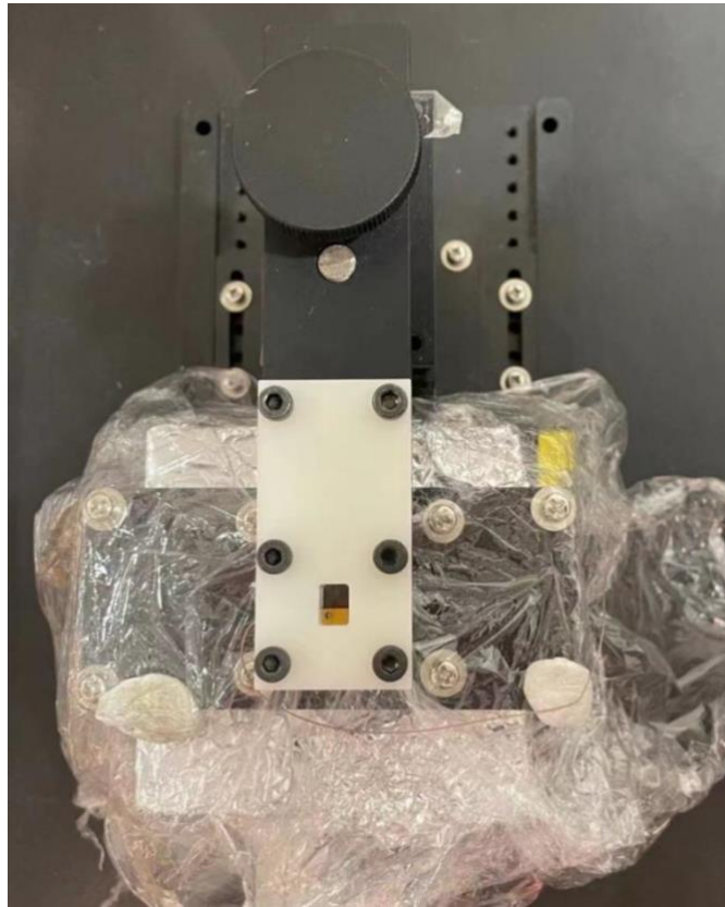
Figure 2.3 The setup of flexoelectric coefficient measurement for U and N bending. The cantilever bending method is used to measure the effective transverse flexoelectric coefficient.
