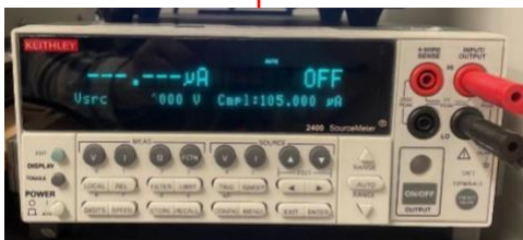
Figure 2.5 The setup of photocurrent measurement to test the photovoltaic effect. The data due to the photovoltaic effect is collected by KEITHLEY 2400 source meter.
