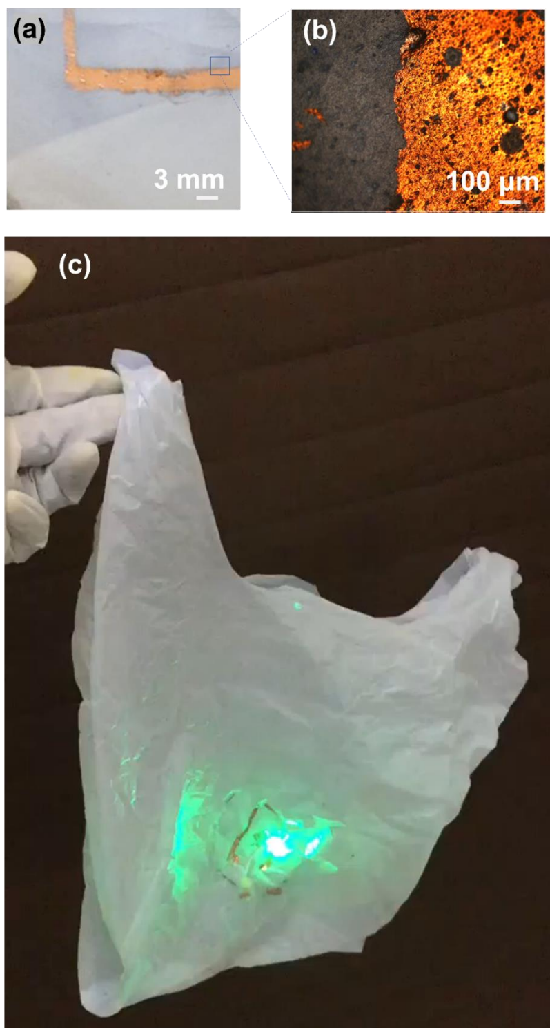
Figure 6.13. a) Optical photo of the inkjet-printed Cu electrode on a plastic bag. b) Optical microscopic image of the enlarged view of the surface of the xerogel-based Cu electrode on the plastic bag. c) Optical photo of the inkjet-printed circuit on a plastic bag forming a closed loop that can power a LED light.
