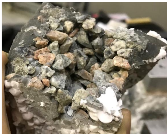
Figure 6.11 Inefficient penetrability of grout in PAC
