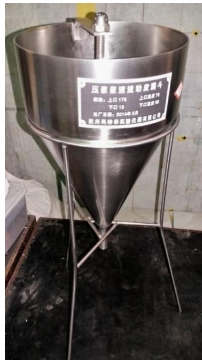
Figure 3.9 Flow cone test setup
