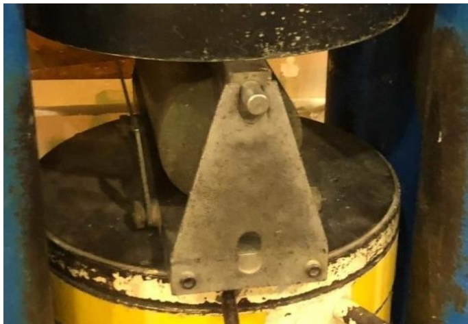
Figure 3.14 Splitting tensile test setup
