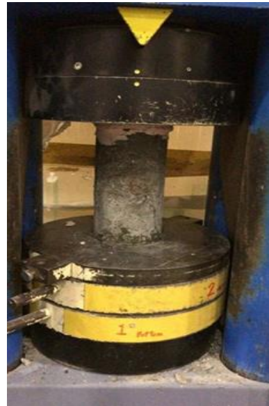
Figure 3.13 Compression test setup
