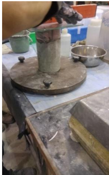
Figure 3.12 Capping of cylinders
