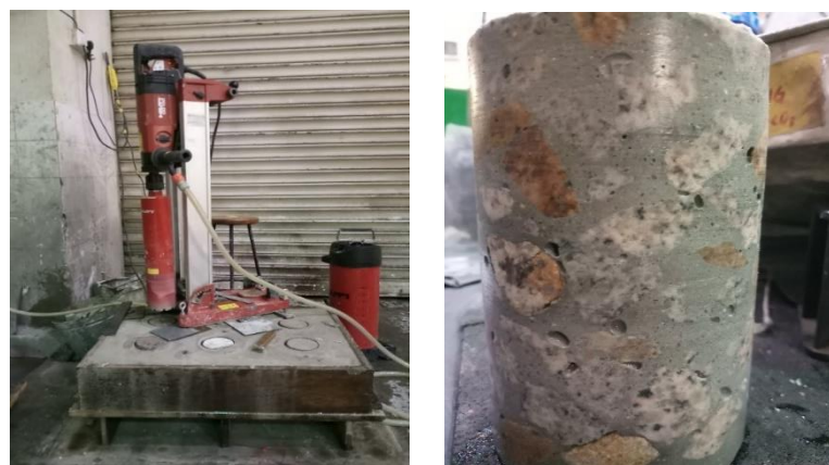
Figure 3.17 Drilled cores for estimation of excess voidage
