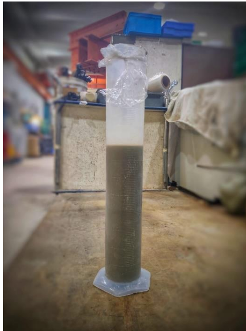
Figure 3.10 Bleeding of grout
