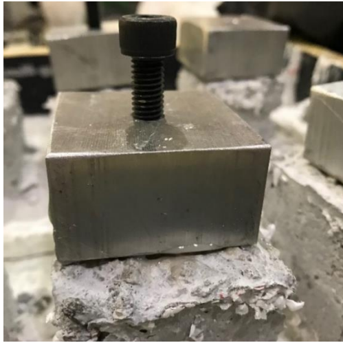
Figure 6.5 Metal block attached to repair material
