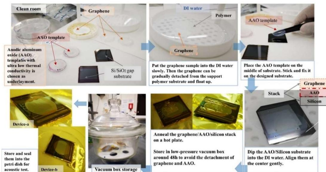
Fig. 6.7: Procedures of graphene thin-film layer transfer onto a prepared substrate (50- $\mu\text{m}$  gap Si/SiO<sub>2</sub> substrate with AAO template) in the in-house Cleanroom.
