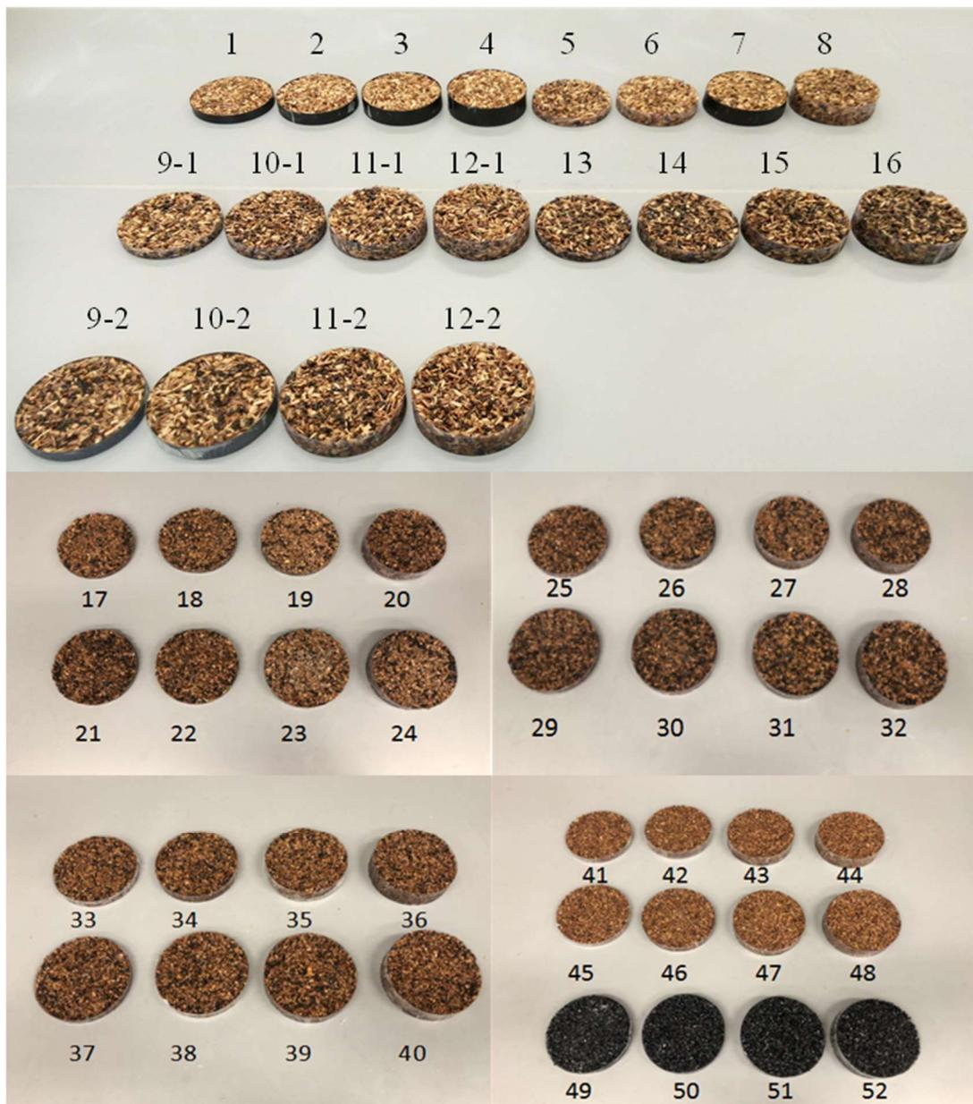
Fig. 4.5: Test samples of wood-rubber composite materials.
