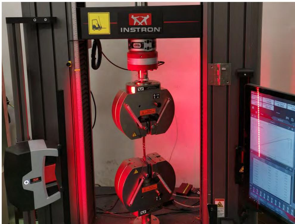
**Figure 5.9** The universal testing platform used in the tensile test.
