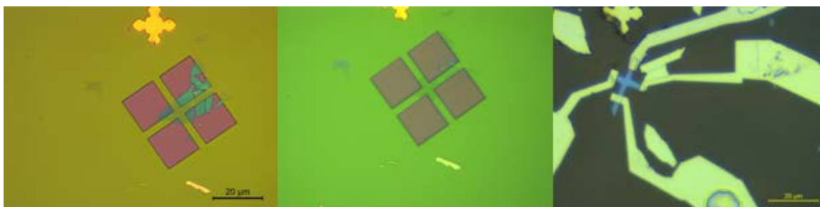
Figure 3.5 (a) Hall structure before etching, (b) after etching, (c) fabricated flexible BP device.
