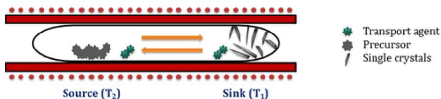
Figure 3.1 Schematic diagram of CVT.[67]
