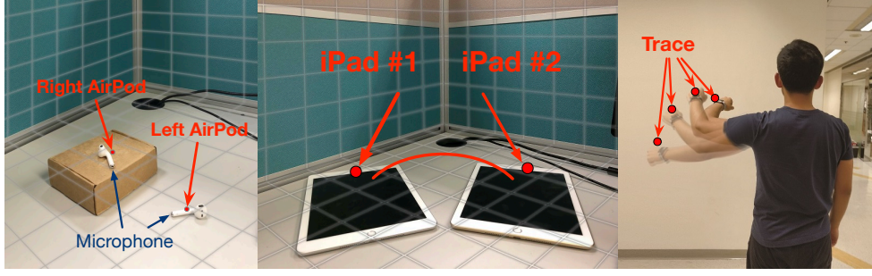
Figure 6-24: UPS+ in real-world applications. (a) shows how UPS+ enables finding the wireless headphone (e.g., AirPods); (b) shows how UPS+ enables pairing two tablets (e.g., iPads); (c) shows how UPS+ enables tracking hand arm through a wearable (e.g., Apple Watch).
