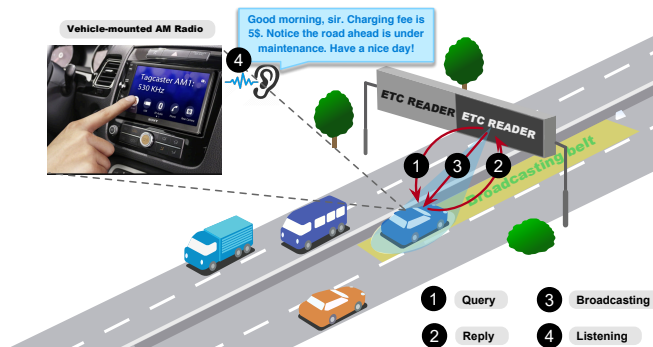
Figure 5-1: Tagcaster-enhanced wireless voice service for ETC system. ❶ The ETC reader queries the transponder attached on the vehicle. ❷ The transponder is identified through its reply. ❸ Tagcaster broadcasts the wireless voice to the identified vehicle. ❹ The driver can listen to the AM radio through the vehicle-mounted radio receiver.
