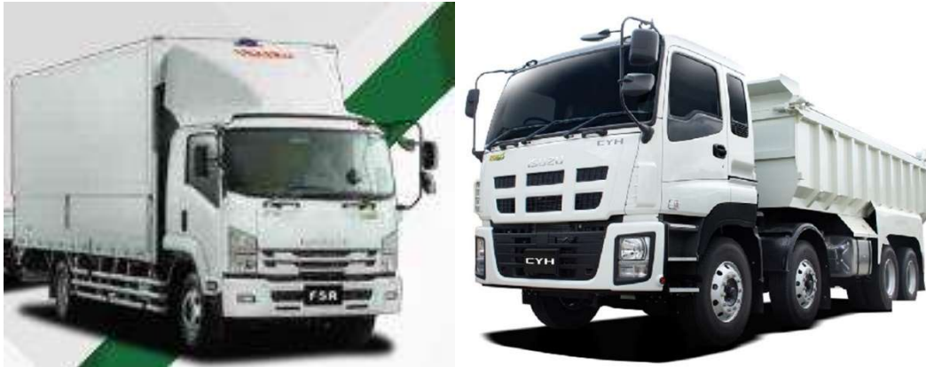
Figure 3.32: A medium goods vehicle: Isuzu FSR90 (the left one) and a heavy goods vehicle: Isuzu CYH52 (the right one), the Length/Width/Height are 7.875m/2.20m/2.53m and 10.66m/2.49m/2.98m respectively ( https://www.isuzu.com.hk/index-cn )
