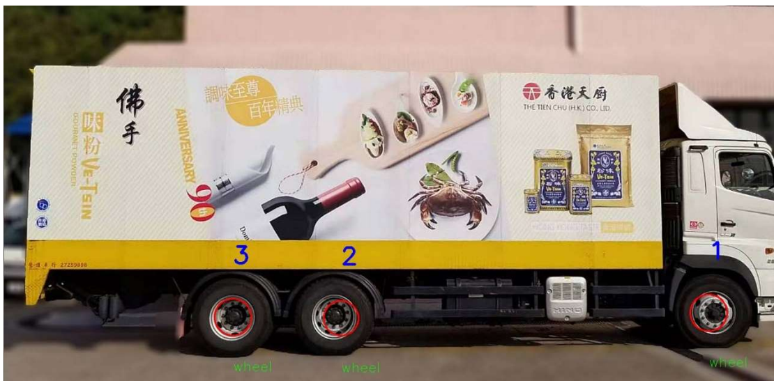
Figure 3.37: Wheel counting after applying the Hough transform algorithm
