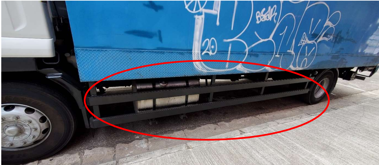
Figure 4.15: Sideguard installed in a goods vehicle
