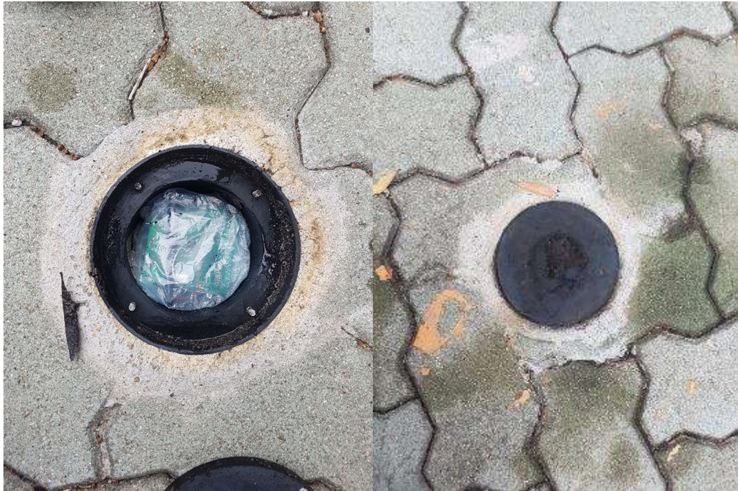
Figure 4.7: Geomagnetic sensor placed into a mounting case, view without a cover (Left) and view with a cover (Right)
