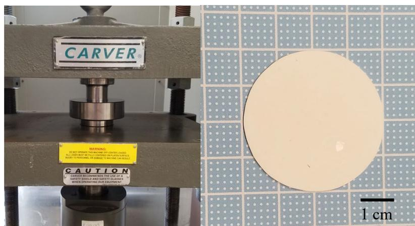
**Figure 3.3** The picture of matching layer under an 8 tons weight in a custom designed mold (Left) and the cured matching layer after the compression (Right).
