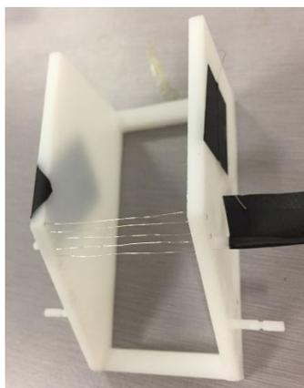
**Figure 5.9** Picture of the tungsten wires holder.
