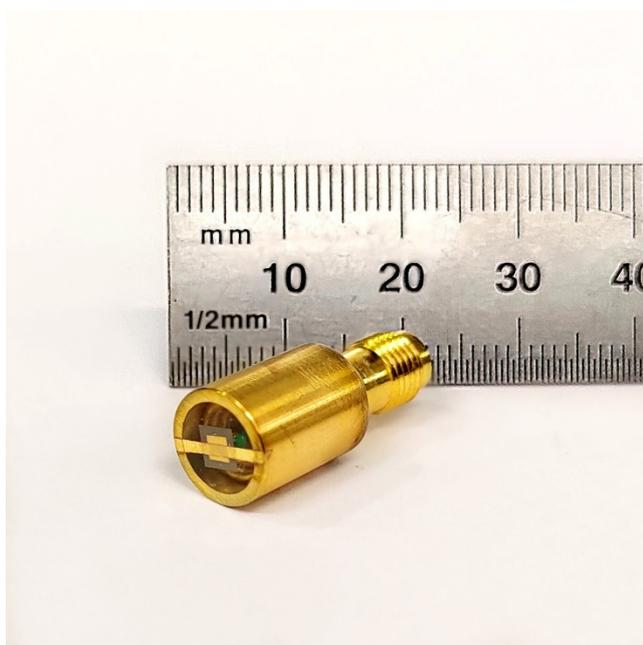
**Figure 3.9** The picture of the single element ultrasound transducer attached with the high pressure compressed matching layer.
