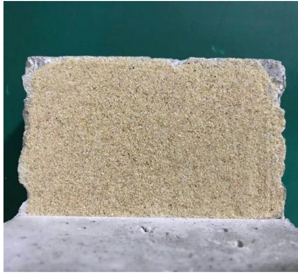
(c) Sand-filling of the rough surface
