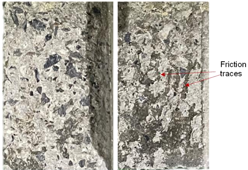
(c) Specimen with applied compressive stress (Specimen O20-N40-R0-S1.5- II )
