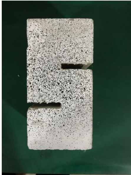
Figure 4.13 Surface preparation of a specimen for DIC measurement
