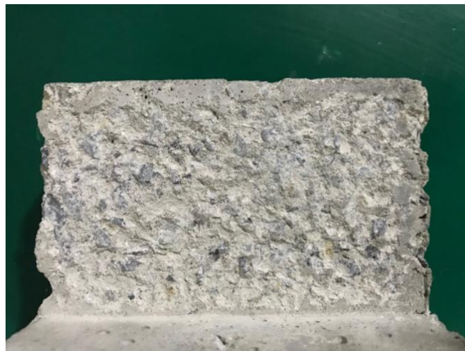
(b) Chisel-roughened surface
