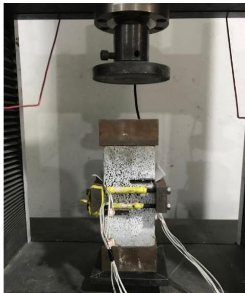
(b) Specimen ready for testing
