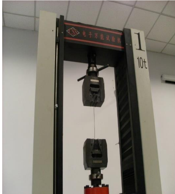
Figure 4.9 Tensile test on the steel bar with 4 mm diameter
