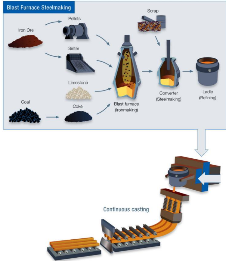
Figure 2 Blast Furnace-Basic Oxygen Furnace (BF-BOF) production route (Source: Eurofer)
