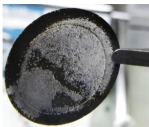
**Figure 6.17** Optical photo of Na deposition on Sn-coated separator with 4 mAh/cm<sup>2</sup> at 1 mA/cm<sup>2</sup>.
