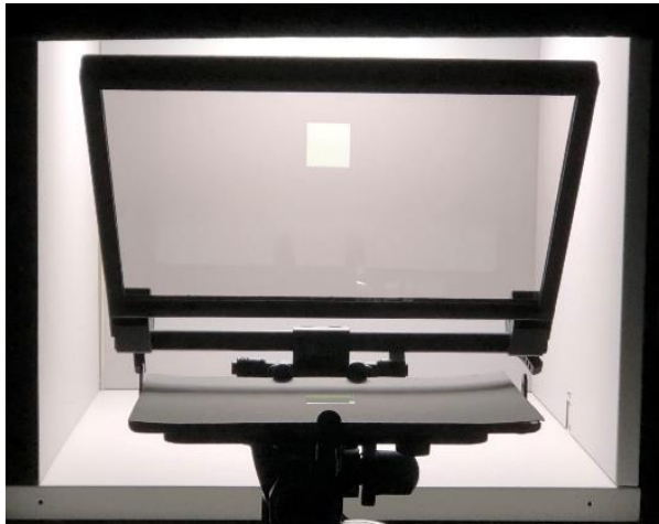
Fig. 6.2. Photograph of the experiment setup, showing the condition viewed by an observer. The stimulus was projected from the iPad display through the beam splitter and was viewed by the observers perpendicularly with an FOV around 4°.
