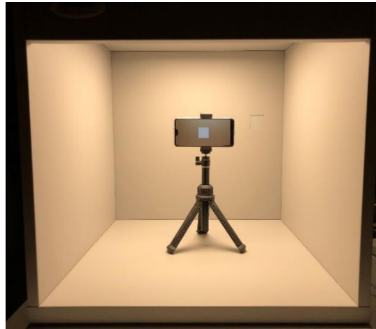
Fig. 6.6. Photograph of the experiment setup. The stimulus was a 3-D cube produced by a customized Unity application and was viewed by the observers perpendicularly with an FOV around 3°.
