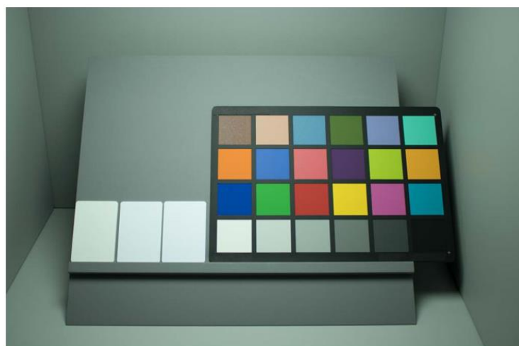
Fig. 4.1. Photograph of the experiment setup, which was captured under the illuminant containing a normal level of UV/violet radiation.
