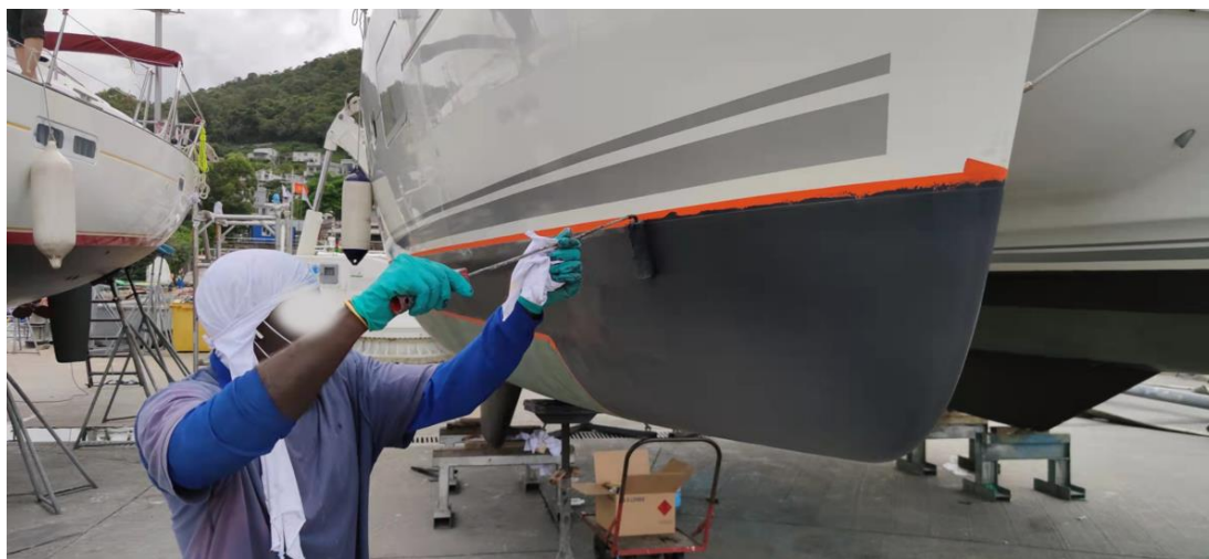
Figure 1.4. Application of antifouling paint to a boat hull.
