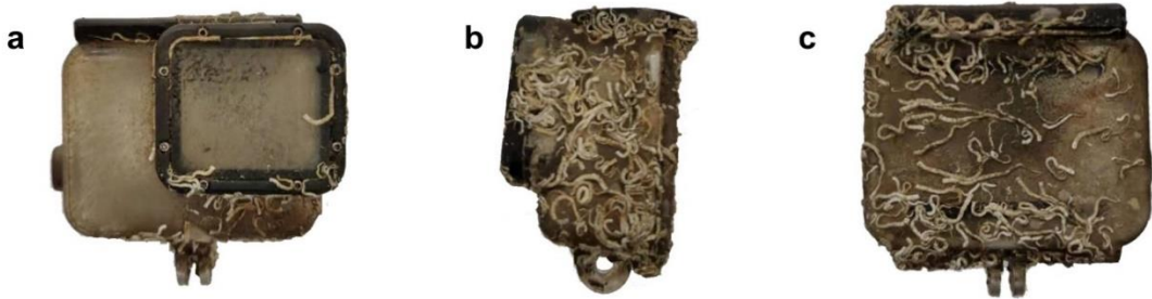
Figure 3.1. An underwater camera cover after one-month submersion in the ocean. (a) Front, (b) lateral, and (c) back views.
