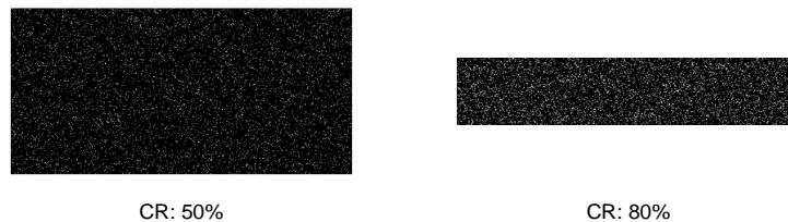
Fig. 5.1. Measurement matrices with CR of 50% and 80%.
