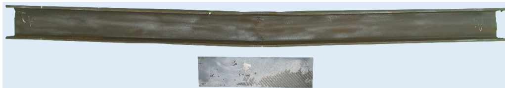
Fig. 7-7 Typical failure mode of BP300 beam series at various temperatures.
