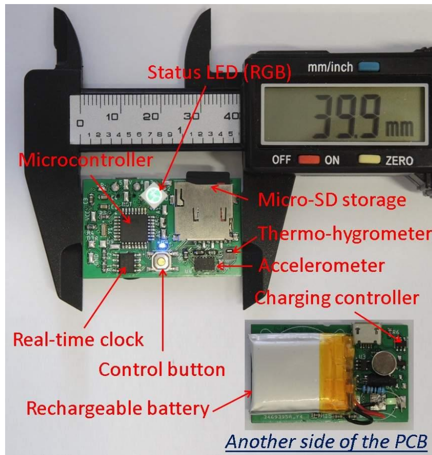
Figure 5.13. Illustration of the PCB used in the sleep position device.
