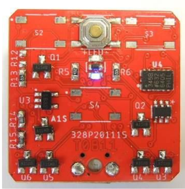
Figure 5.6. The printed circuit board of the control box.
