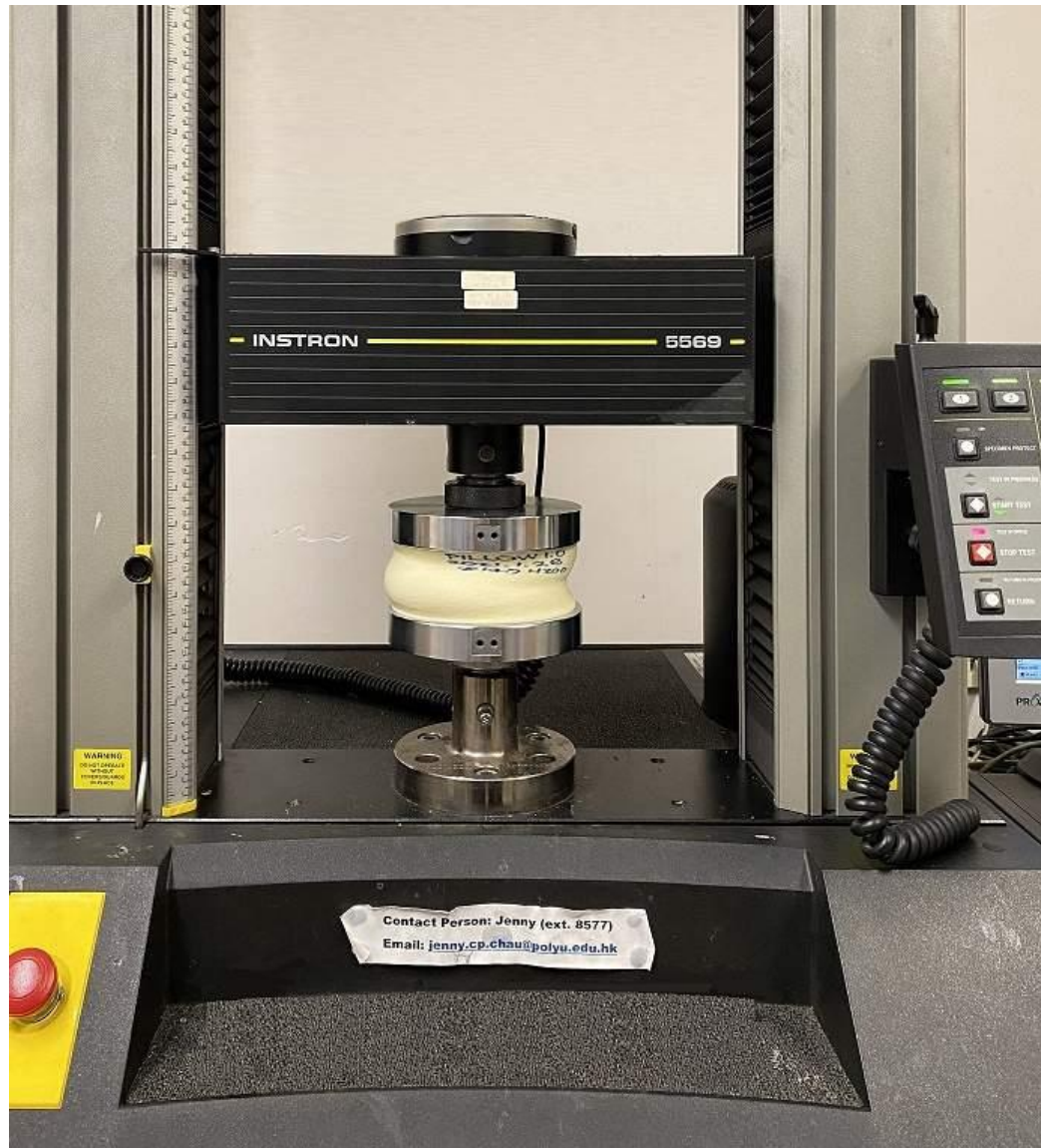
Figure 3.47. The material test machine and a specimen being tested.
