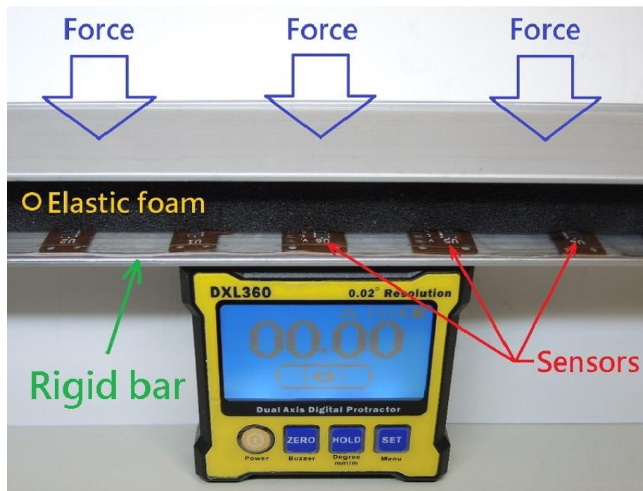
Figure 3.28. Design of the sensor tape calibration.
