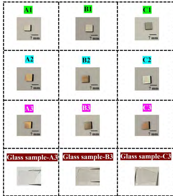
Figure 5.15 Photographs of the annealed coated (Ru–Cr) samples and tested glass specimens.
