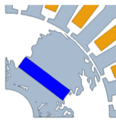
(b) Model 1 T_{avg}=2.57Nm T_{ripple}=0.85Nm
