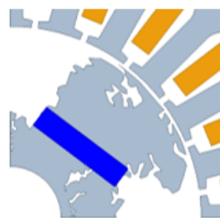
(a) Model 0 T_{avg}=2.41Nm T_{ripple}=0.38Nm
