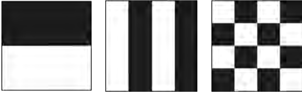
Figure 2-6 Examples of different textures: Each image above has a 50%-50% distribution of black and white pixels but of different textures (Wirth, 2004)
