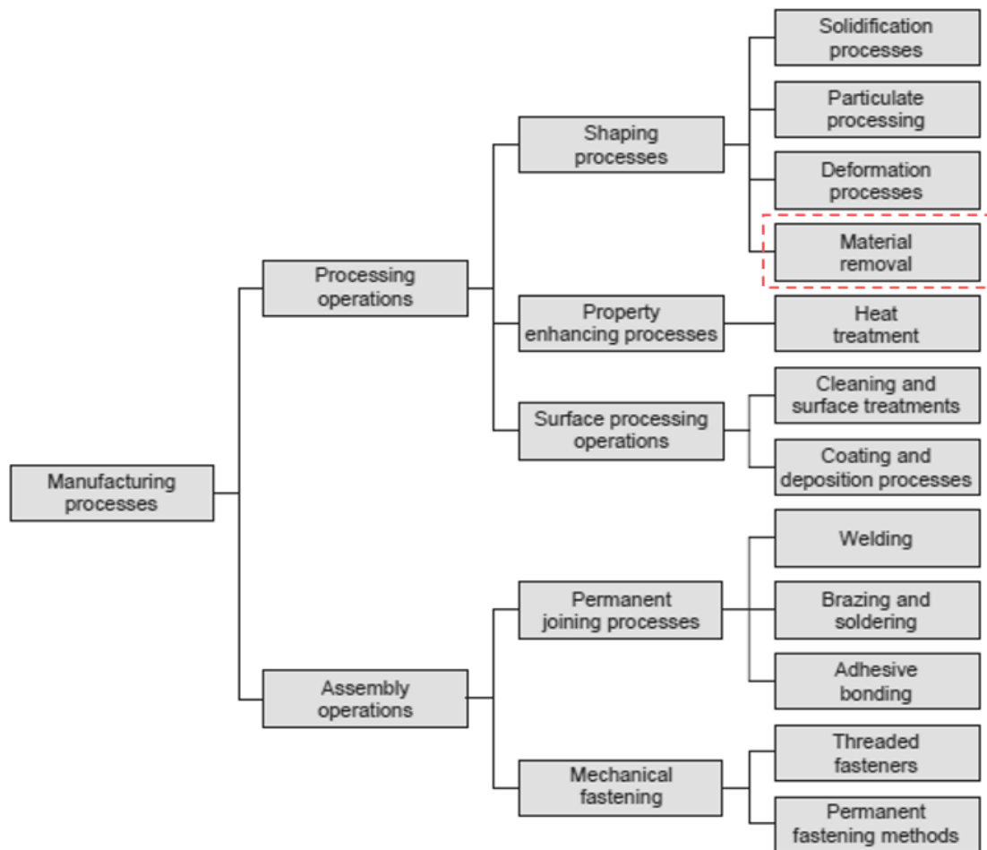
Figure 2.1 Classification of manufacturing processes (Groover, 210AD).
