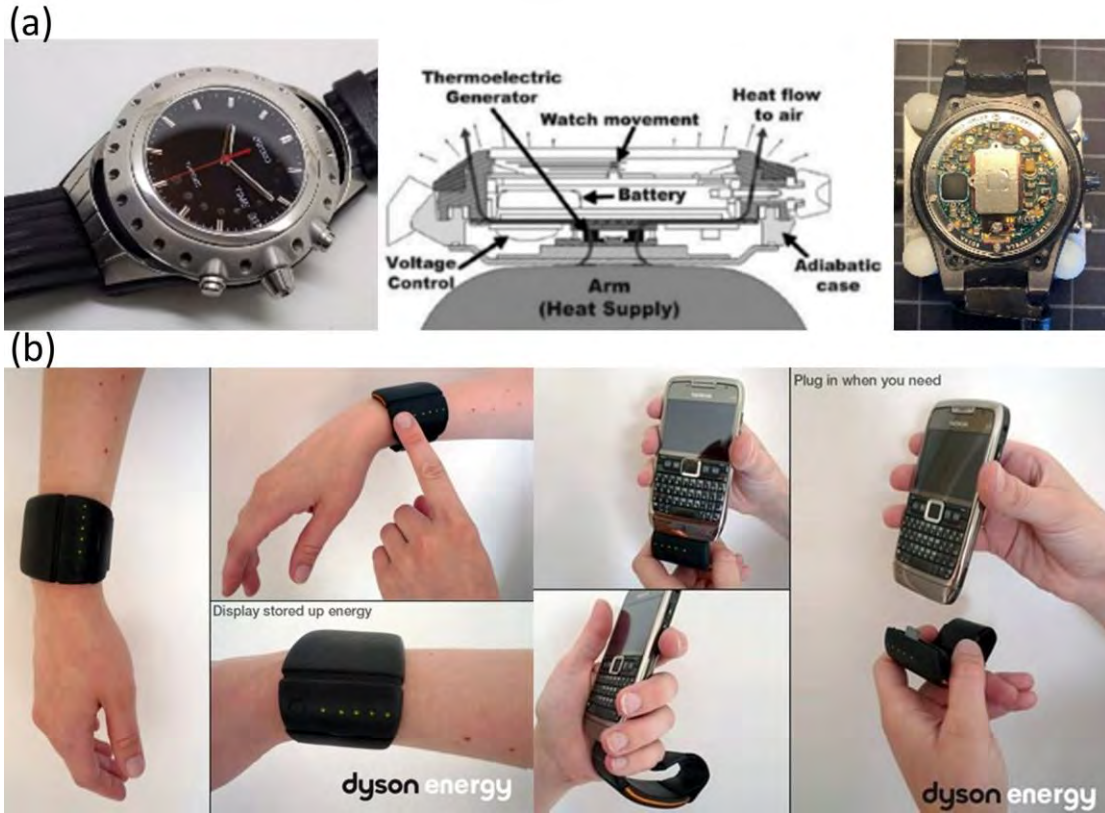
Figure 2.14 Photo of (a) body heat powered watch Seiko thermic 196 (b) Dyson energy bracelet. 197
