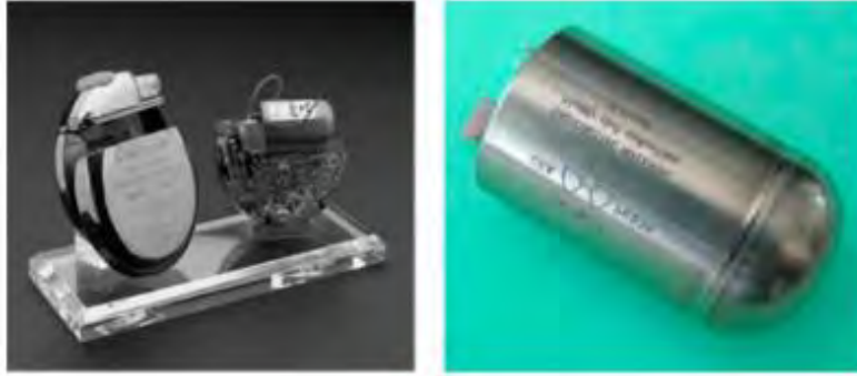
Figure 2.17 Pacemaker(left) and RTG battery(right). 209
