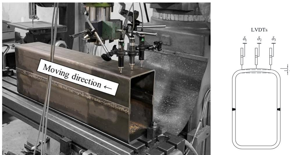
Figure 4.7 Instrumentation of the local imperfection measurement.
