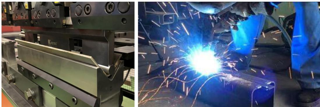
Figure 2.3 Manufacturing process of press-braking RHS tubes.
