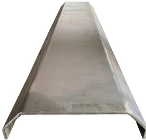
Figure 5.1 Half section of irregular octagonal hollow section ( $H/W = 2$ ).
