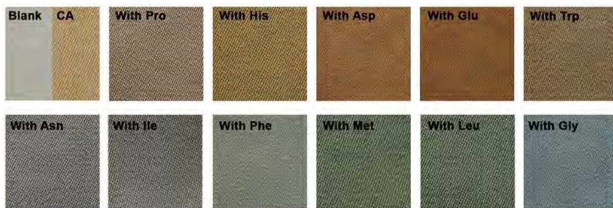
Figure 4.8 The photographic images of the dyed wool fabrics: (a) Blank; (b) CA only; (c) CA with Pro; (d) CA with His; (e) CA with Asp; (f) CA with Glu; (g) CA with Trp; (h) CA with Asn; (i) CA with Ile; (j) CA with Phe; (k) CA with Met; (l) CA with Leu; (m) CA with Gly
