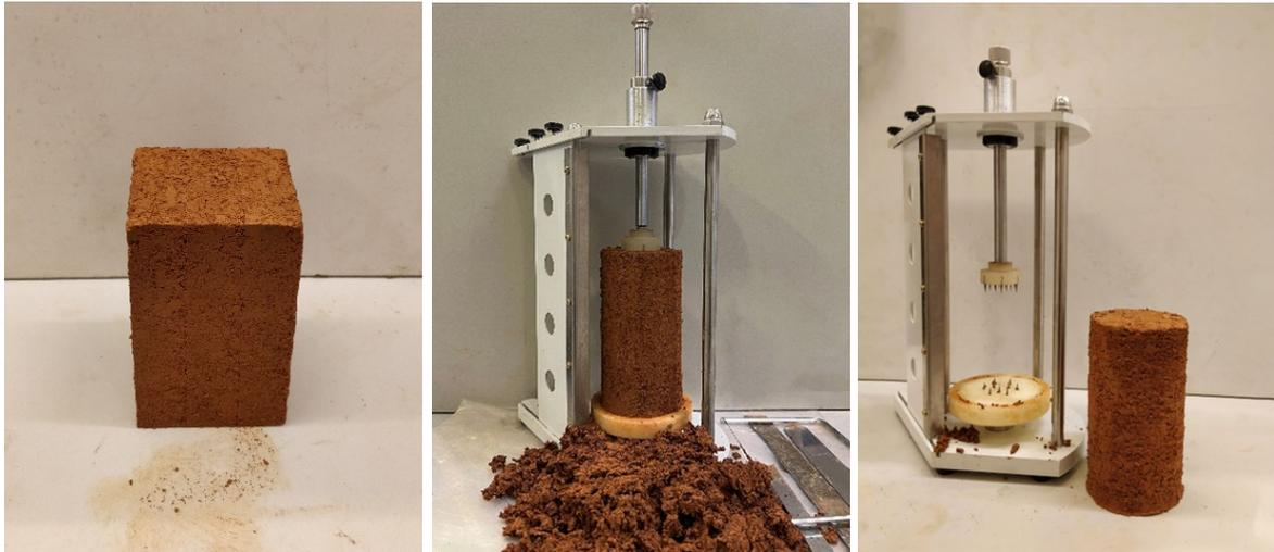
Plate 3.3 Carefully trimmed horizontal cut specimen
