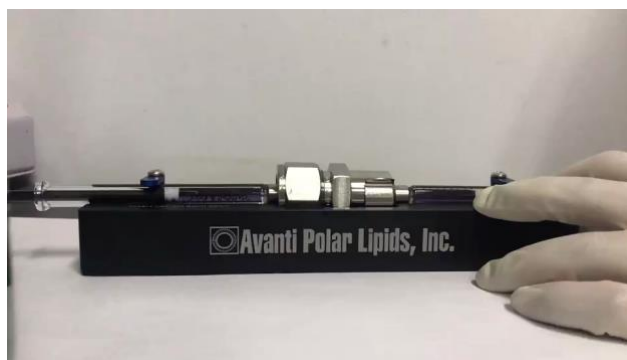
Figure 19. The process of extrusion by Avanti Polar Lipids.
