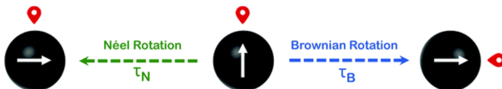
Figure 31. Illustration of the magnetic relaxation mechanisms in MNPs. Image modified from Ref. [68].
