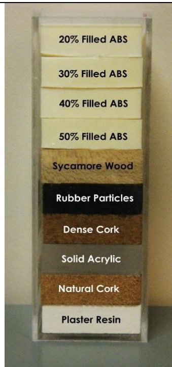
Figure 3. The Credence Cartridge Radiomics phantom with 10 cartridges for radiomic feature robust analysis against scanners, image acquisition protocols, and reconstruction algorithms. Each cartridge contains unique textures. The top four cartridges are 3D printed ABS plastic with 20% to 50% honeycomb fill, which provide regular and periodic textures. Then, the following cartridges are sycamore wood, cork, extra dense cork, solid acrylic, natural cork, and plaster resin. The lower six cartridges provide natural textures for the radiomic. The image is adapted from TCIA [24].
