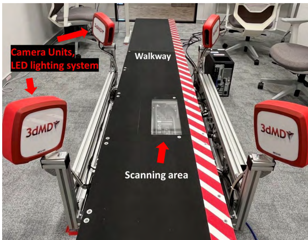
Figure 4. 1 Setup of 4D foot scanning system.
