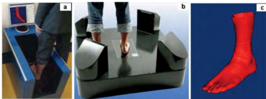
Figure 2. 10 (A) 3D laser scanner; (B) FotoScan scanner; (C) 3D foot model using 3D scanner[100]
