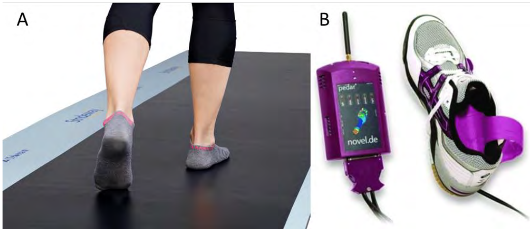
Figure 2. 6 Foot-pressure monitoring system (A). Modular platform, Strideway System (B). Pedar insole system[76]
