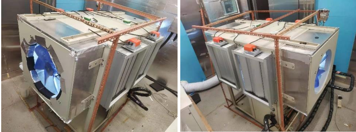
Photo 1 The novel DFOC of the experimental ASHP / DFOC unit
