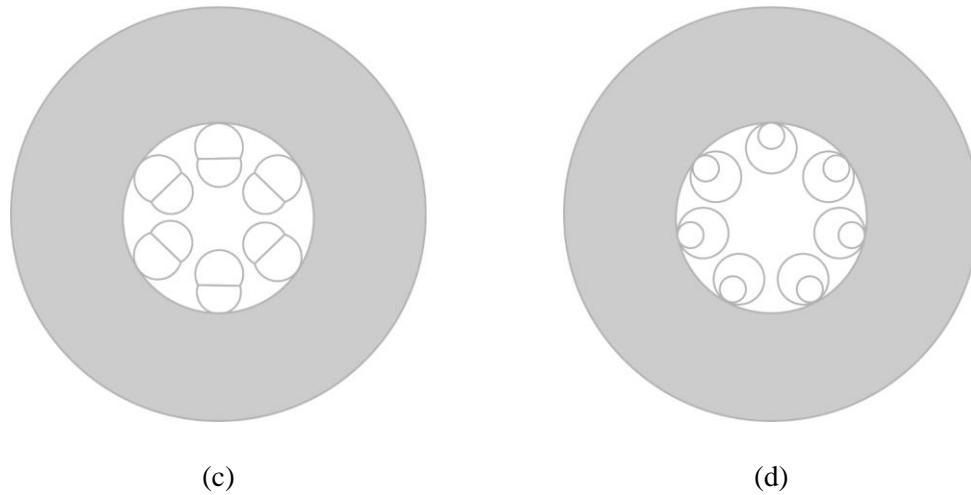
Fig. 2.9 Schematic diagram of HC-ARFs. (a) Kagome HCF. (b) Single-ring HC-ARF. (c) HC-CTF. (d) HC-NANF.
