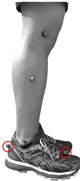
Figure 3.1. Marker model used for detection of foot-strike pattern.
