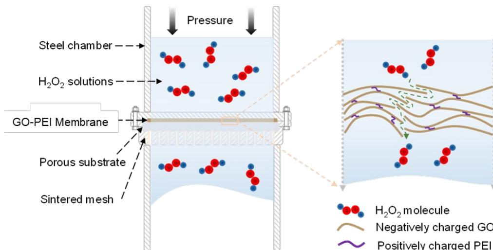
Fig. 4.6 Schematic drawing the transport of H<sub>2</sub>O<sub>2</sub> through anti-swelling GO-PEI membranes
