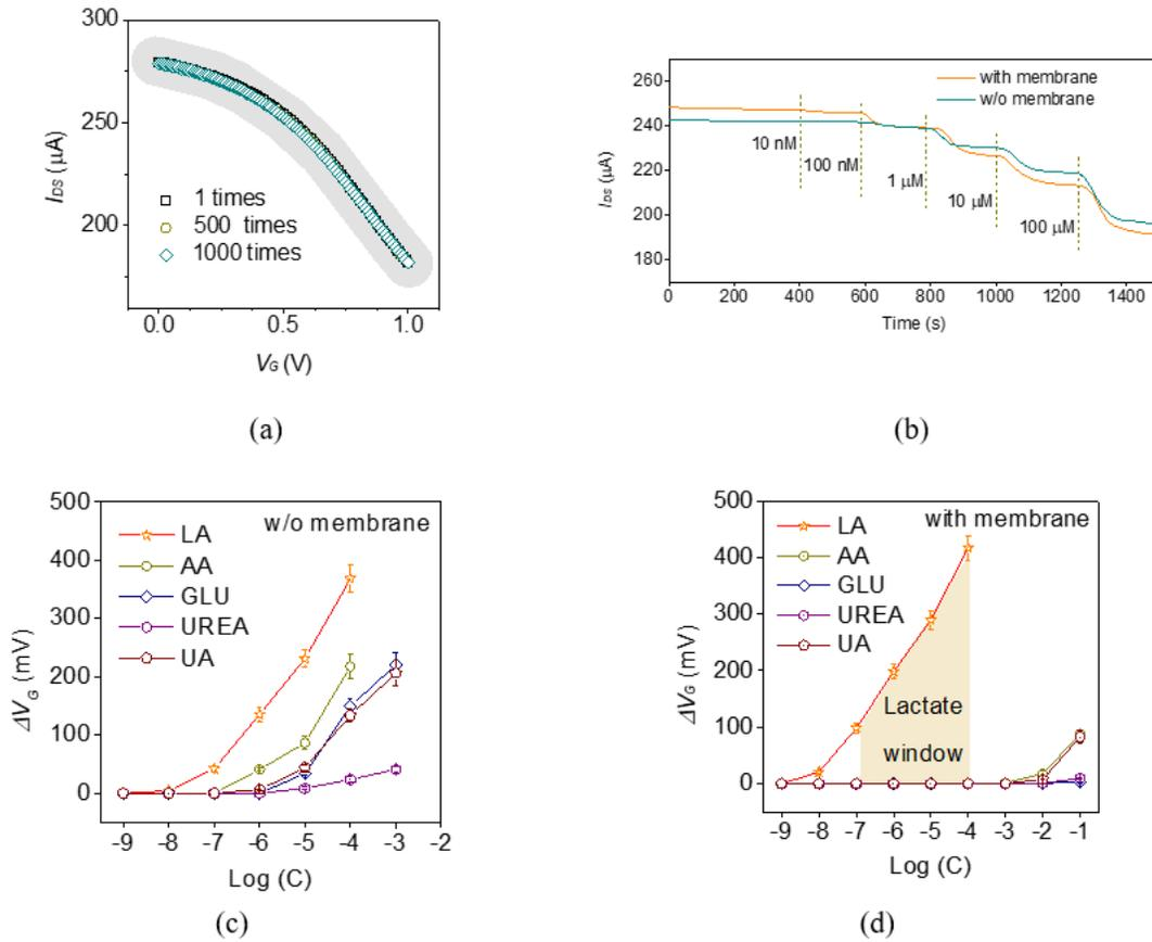
Fig. 4.9. (a) The transfer characteristics of an OECT measured in PBS solution after the repeated tests up to 1000 times. (b) The response of OECT to lactic acid and lactate oxidase with and without GO-PEI membrane. (c) The selectivity test without GO-PEI membrane; (d) The selectivity test with GO-PEI membrane
