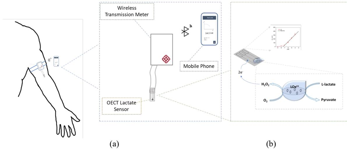
Fig. 5.3: Schematic drawings of (a) wearable sweat-based lactate sensor on Arm; (b) OECT sensor for measuring Lactate concentration
