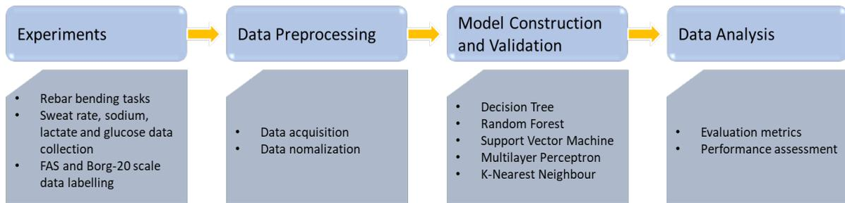
Fig. 3.1. The overall flowchart
