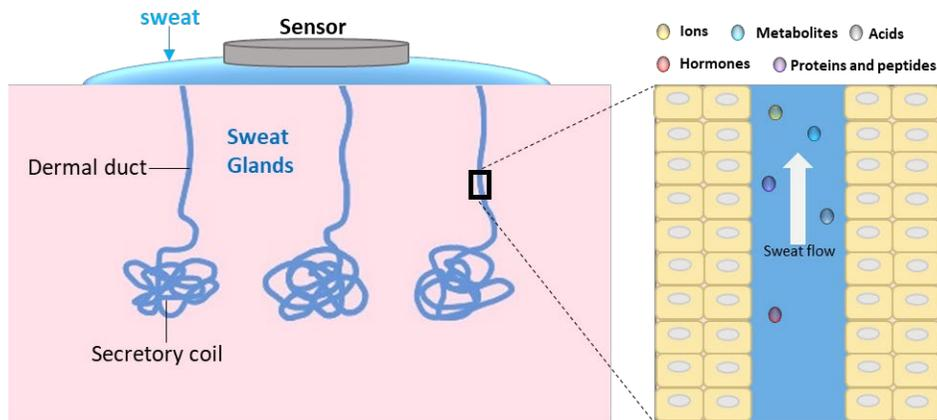
Fig. 2.2 Schematic drawing of sweat gland structure and biomarkers (Bariya et al., 2018)
