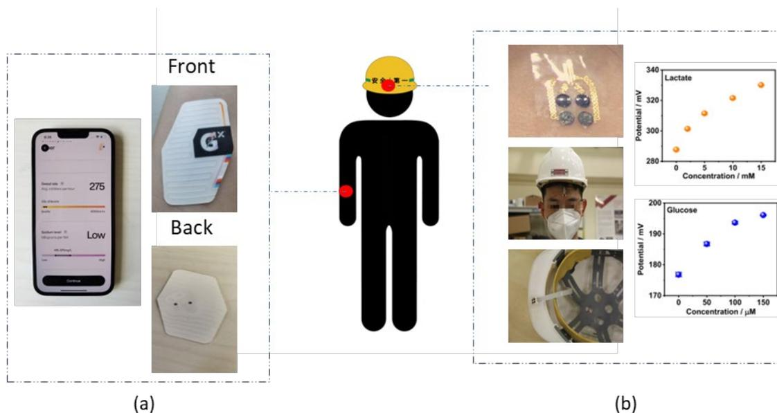
Fig. 3.2. Sweat sensors: (a) Gx sweat patch; (b) the sweat-based lactate and glucose biosensors
