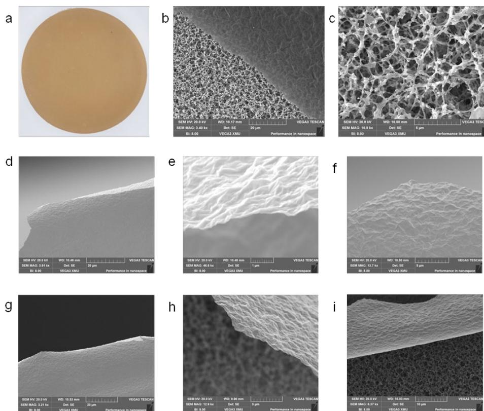
Fig. 4.8. (a-c) Structures of anti-swelling GO-PEI membrane on a porous substrate. (d-f) SEM images of a self-standing anti-swelling GO membrane. (g-i) SEM images of a self-standing anti-swelling GO membrane after soaking-drying in water.
