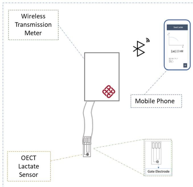
Fig. 4.4. Schematic drawing of wearable sweat lactate sensor
