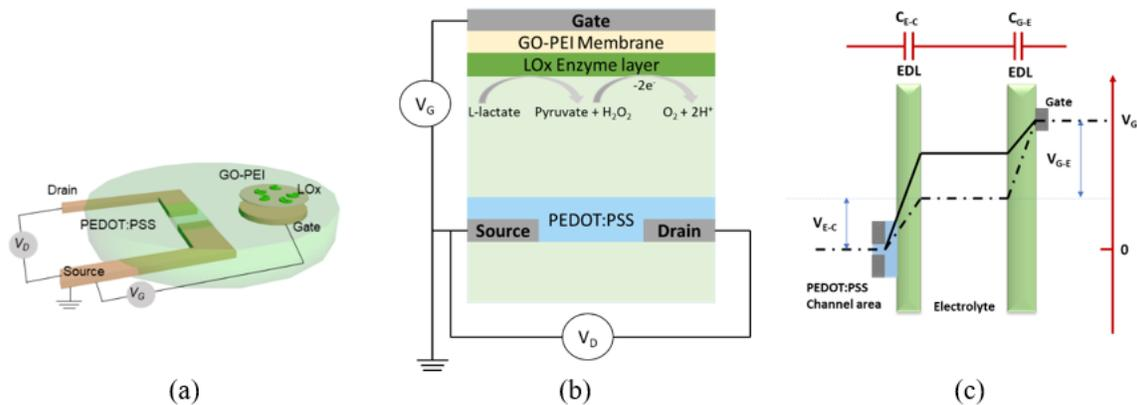
Fig. 4.5. OECT: (a) OECT-based Lactate biosensor Structure; (b) Schematic diagram of an OECT with LOx/GO-PEI membrane/Pt gate; (c) Voltage variations between the gate and channel of the OECT before (dash line) and after (solid line) the addition of Lactate in the electrolyte (Liao et al., 2015b).
