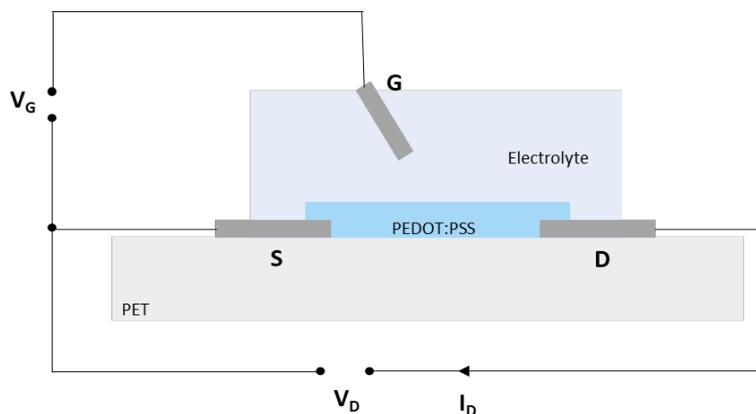
Fig. 4.1. Schematic structure of a typical OEET-based biosensor (Note: G is for Gate; S is for Source; and D is for Drain; IN is for inlet; OUT is for outlet.)
