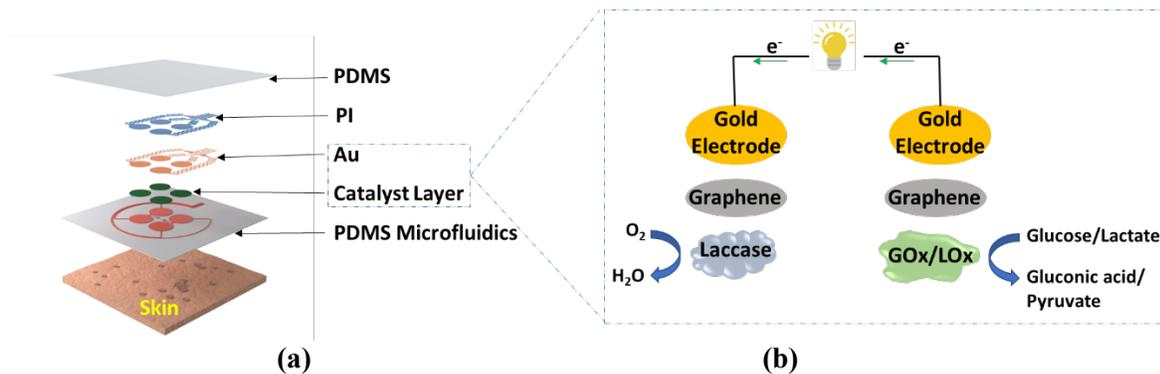
Fig. 3.3. Schematic illustrations of (a) a sweat sensor for measuring lactate and glucose, (b) the mechanism of self-powered biofuel cell
