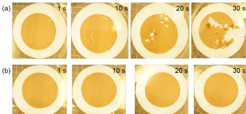
Fig. 4.7. Pictures recording the ultrasonic tests of (a) a GO membrane; and (b) a GO-PEI membrane for 30 seconds.
