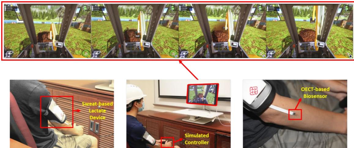
Fig. 5.5. Pictures of construction equipment operation simulation system with on-body Sweat-based Lactate Device
