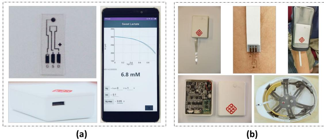
Fig. 6.3. Sweat Lactate Sensor: (a) the three main components; (b) the structure and on-body application
