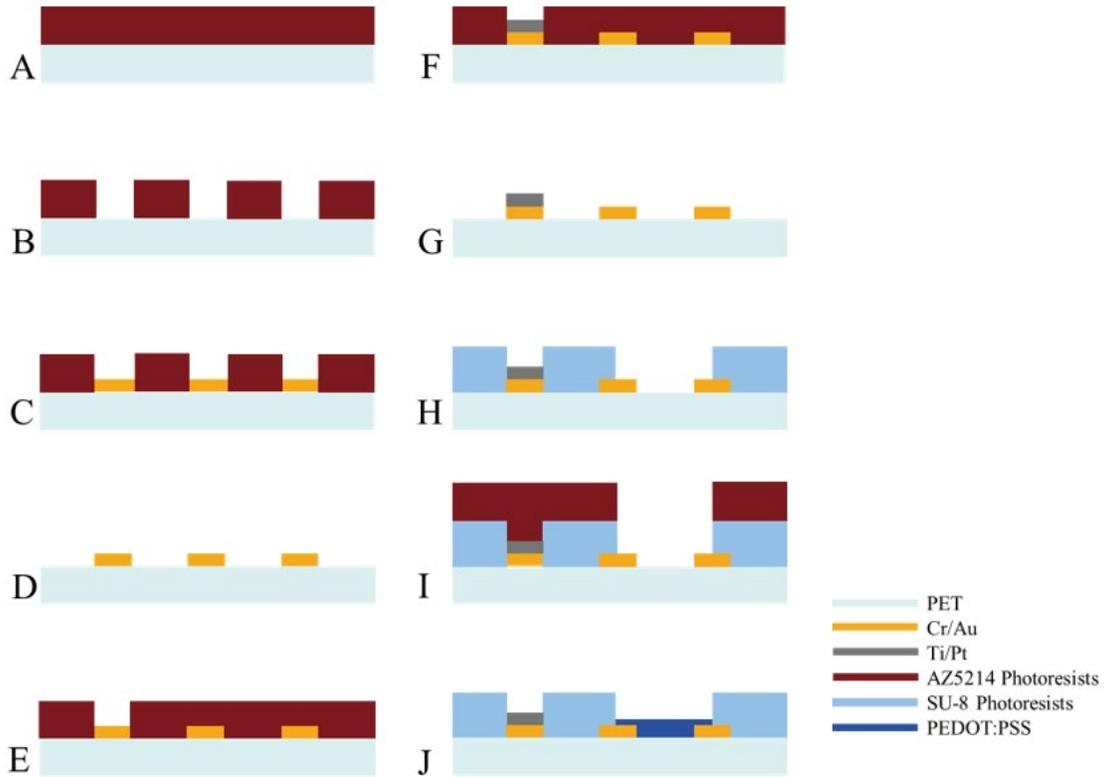
Fig. 4.2. Device fabrication process: (A-D) Cr/Au electrode deposition. (E-G) Ti/Pt electrode deposition. (H) SU-8 photoresists encapsulation. (I-J) Patterning of PEDOT:PSS channel semiconductor.
