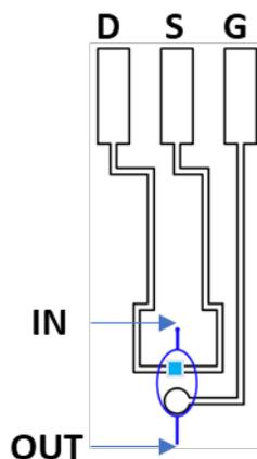
Fig. 4.3. OEET circuit with microfluidic channels
