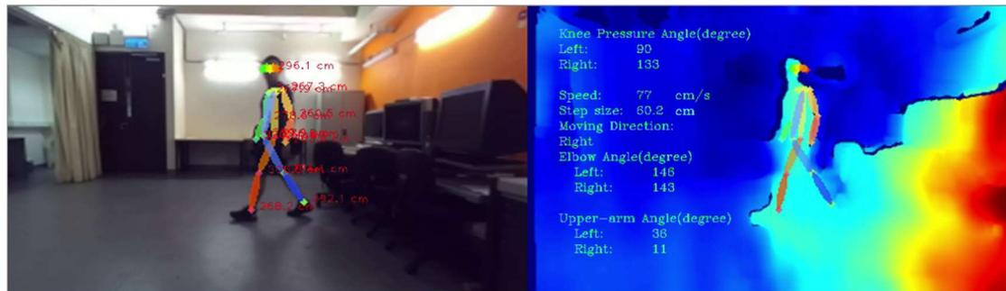
**Figure 5.21** Visualisation of the real-time photogrammetric system for human kinematics
