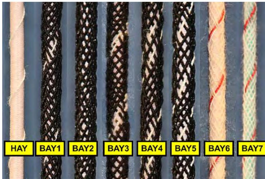
Figure 2.8 The developed braided auxetic yarns and helical auxetic yarn<sup>64</sup>.
