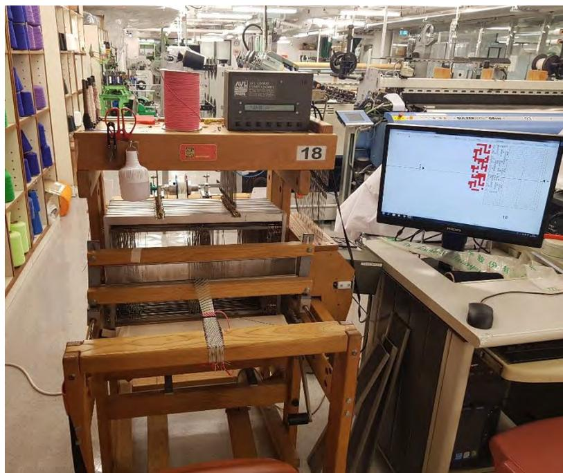
Figure 3.7 Semi-automatic weaving machine used for fabrication.
