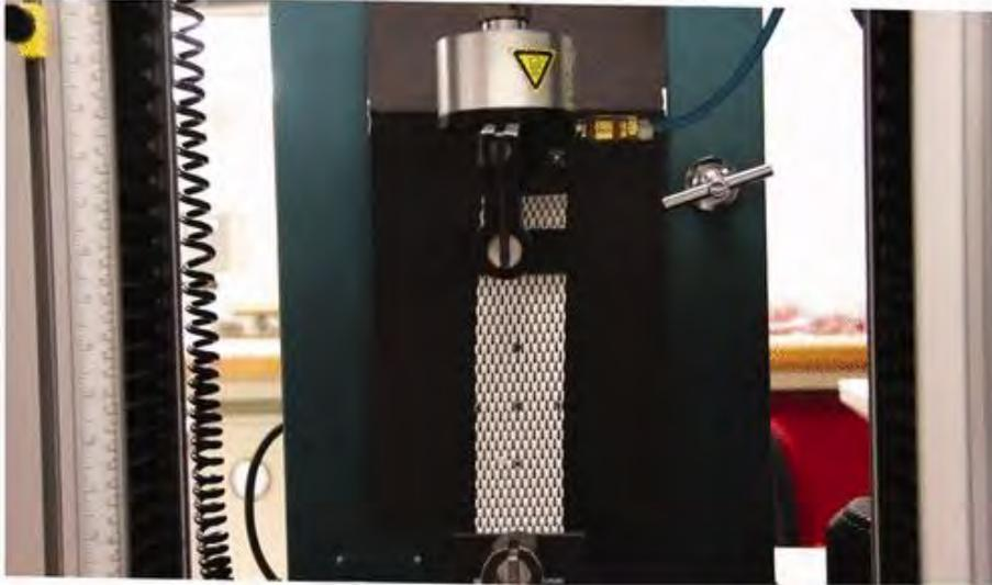
Figure 2.17 Fabric sample mounted on tensile testing machine<sup>39</sup>.
