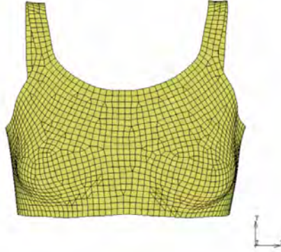
Figure 5.5: FE sub-model of the sports bra.
