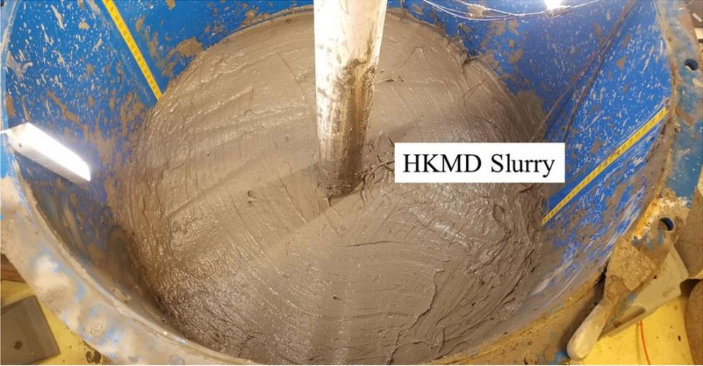
Figure 6.7 Photo after filling the first layer of HKMD slurry
