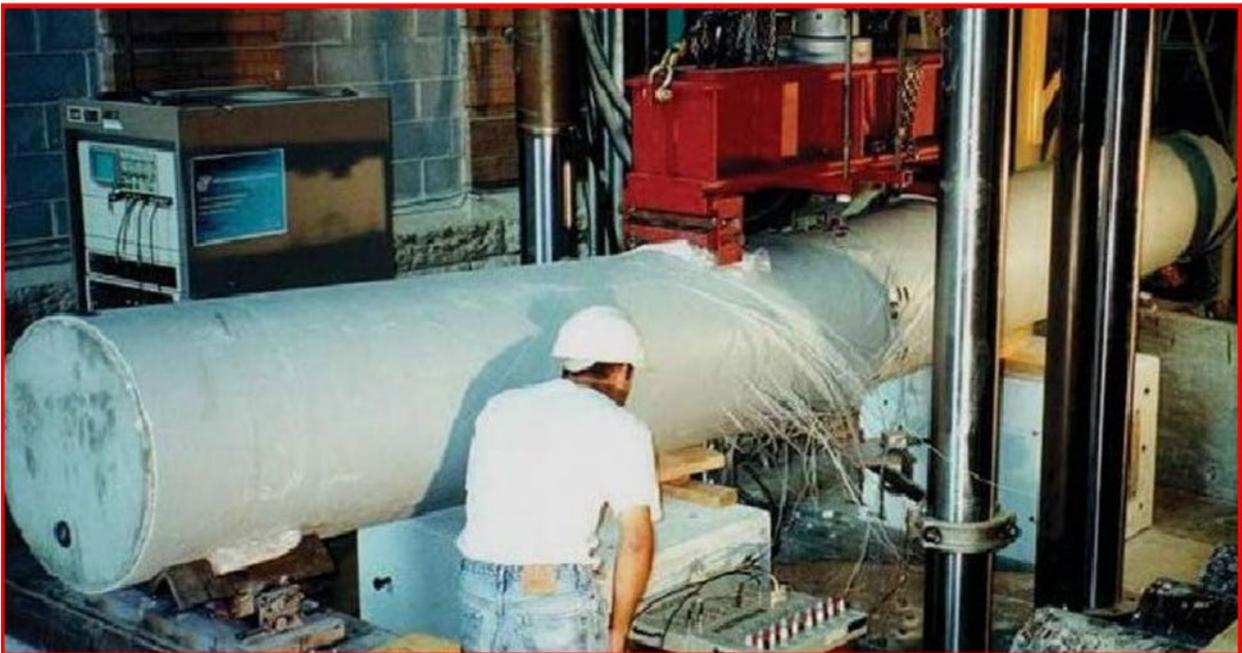
Figure 2.10 Four-point bending test of FRP composite concrete beam (Fam et al., 2003)
