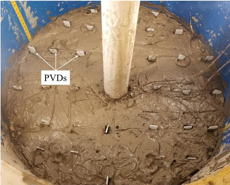
Figure 6.9 Photo after installing the PVDs
