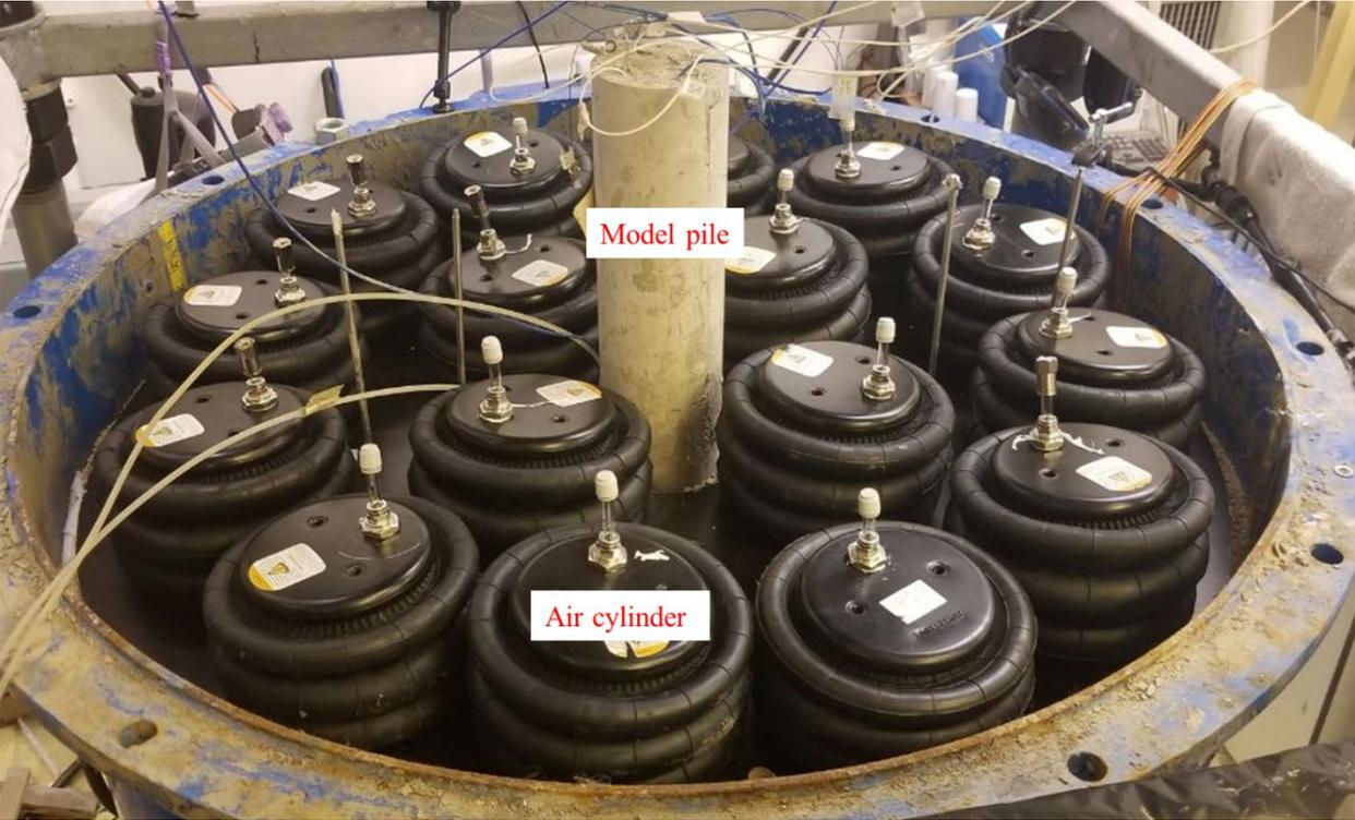
Figure 6.4 Photo of air cylinders layout in the physical model
