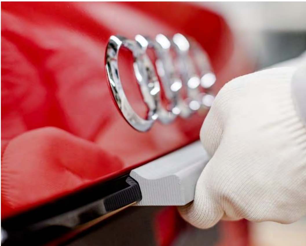
Figure 2.3. Audi 3D-printed products for assembly aid using recycle packaging materials 18 .
