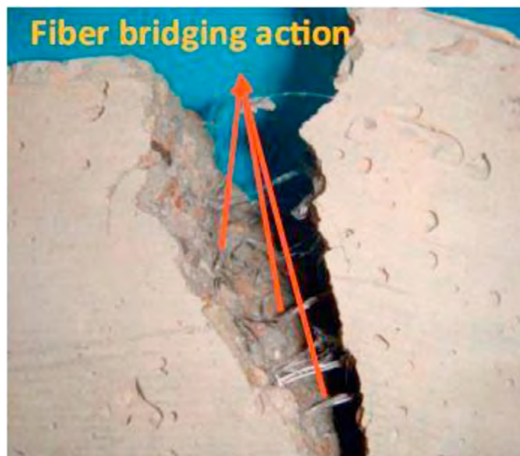
Figure 2.7. Fiber bridging action improving the mechanical properties of concrete 43 .
