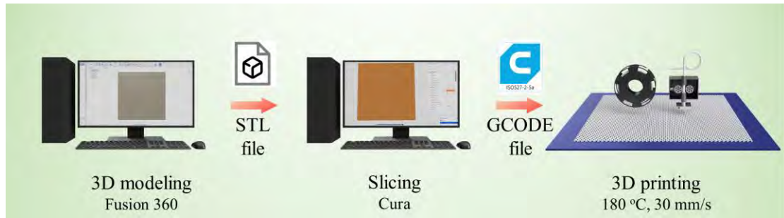
Figure 7.2. 3D printing of rTPU textile samples with program-generated patterns.
