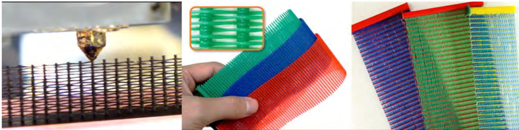
Figure 2.12. 3D-printed woven textiles 75 .
