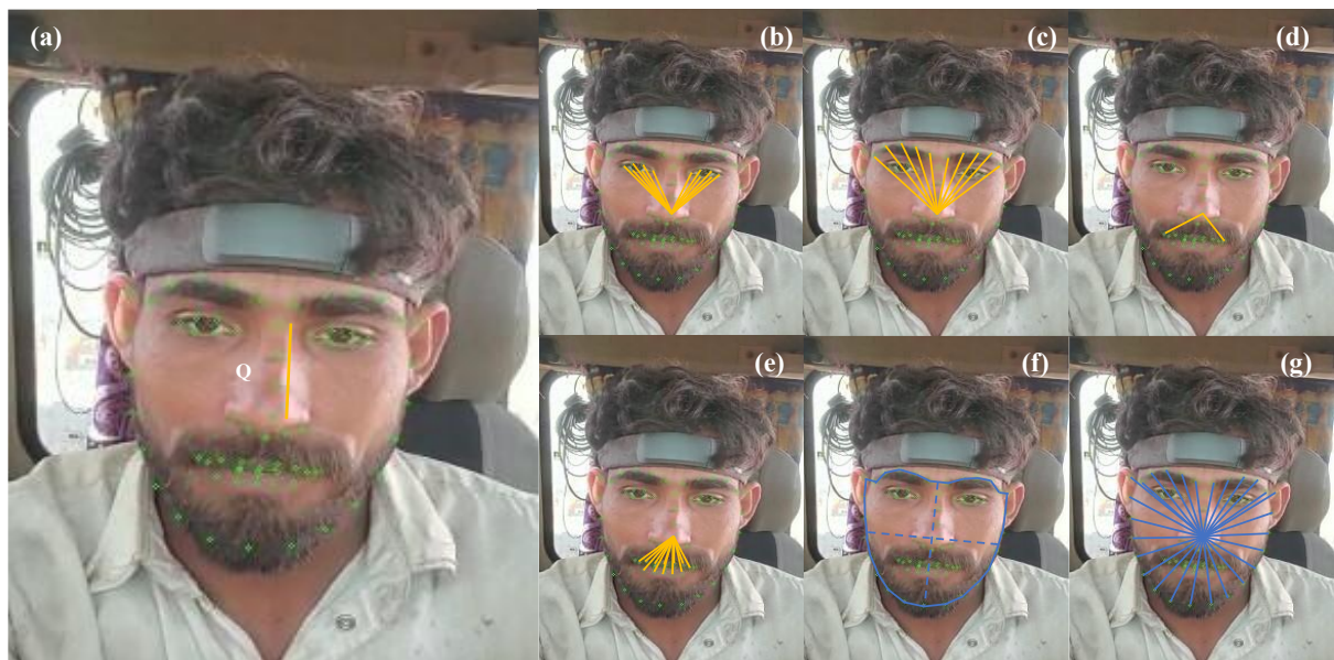
Figure 3.3: (a) identification of facial landmarks and calculation of (b) eye area (c) eyebrow (d) mouth corners (e) mouth outer (f) face area (g) head motion
